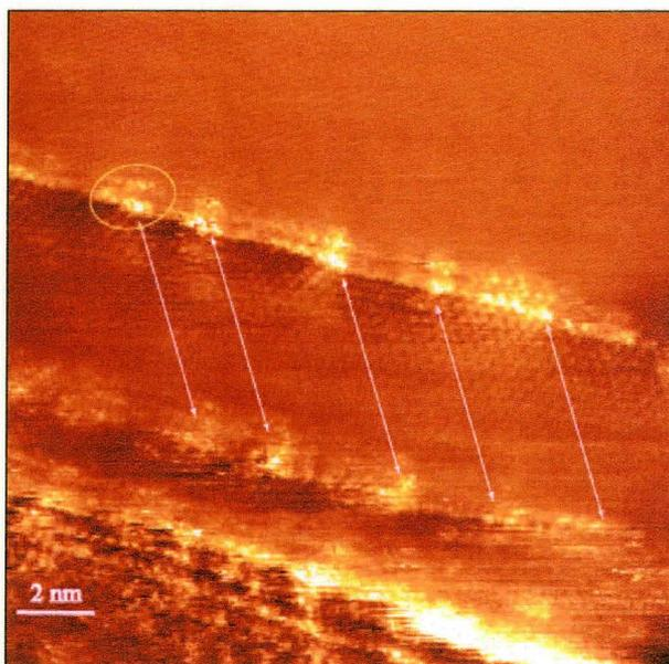
Figure 5-3 The SWCNTs functionalized via the Bingel reaction scan size: 20 nm  $\times$  20 nm.  $V_B = 20.14$  mV.  $I_T = 1$  nA. Scan rate: 19.53 Hz
