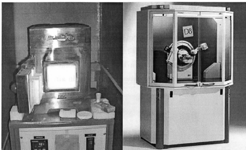
Figure 2.2: High Temperature furnace(left) and X-ray diffractometer(Bruker D8)
