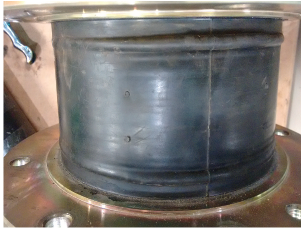
Figure 4.11: Photograph taken after a test with u/t_r = 3 and under \bar{p} = 9 MPa. Excessive rubber bulging is apparent on the top and bottom of the bearing, indicating likely damage in the interior.
