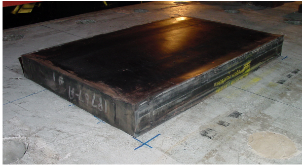
Figure 5.1: Unbonded rubber pad.
