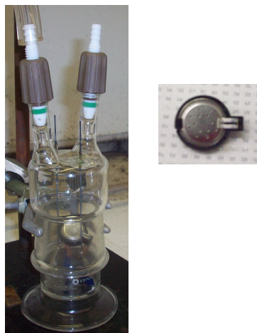
Figure 1-2 (Left) Glass cell chamber which is flooded with pure O_2 gas and housed the M- O_2 cells during electrochemical cycling and (right) a coin cell used to cycle the M- O_2 batteries which had holes drilled in the top to allow O_2 gas to enter the electrochemical system
