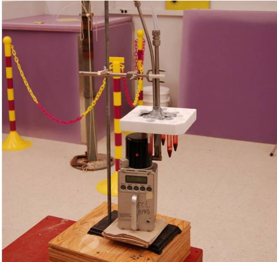
Figure 17. ^{252}\text{Cf} irradiation set-up.
