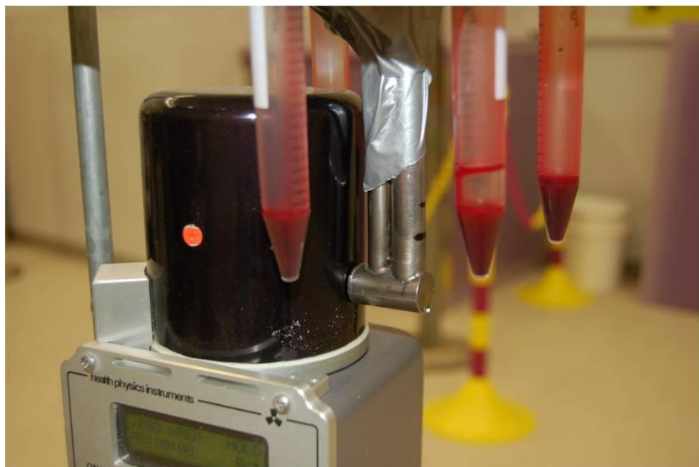
Figure 18. Close-up image of the ^{252}\text{Cf} irradiation set-up.
