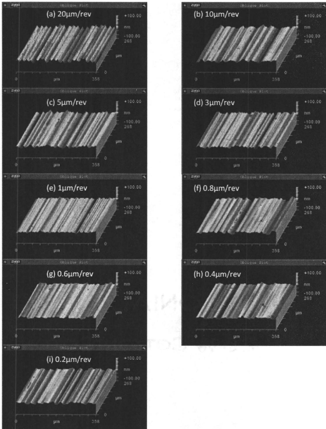
**Figure C-2: 54% cold rolled 99.87% aluminum (1000RPM, 2 $\mu$ m depth, 1.5mm nose radius)**
