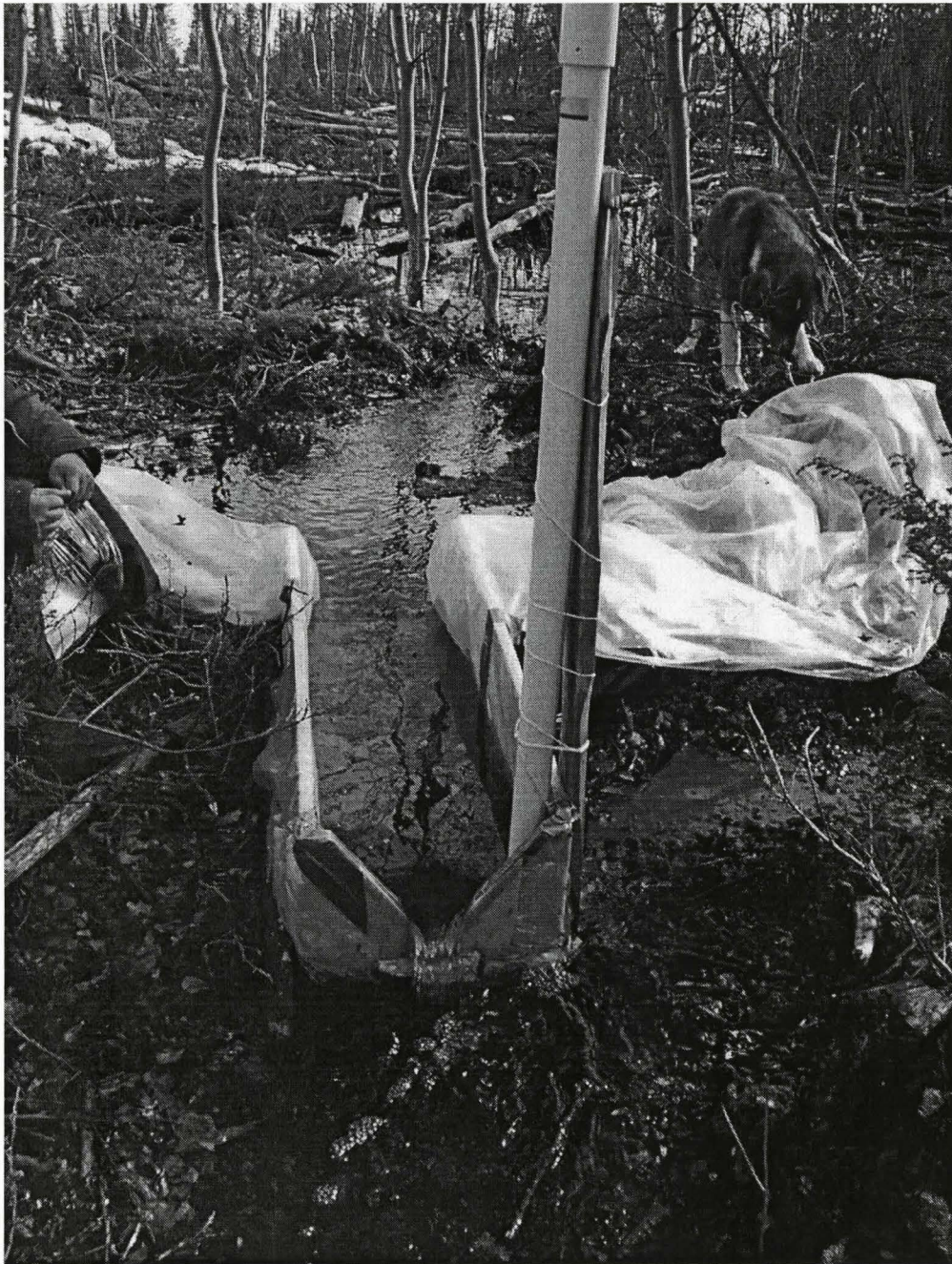
Figure 3.6: Photograph of Experimental slope outlet weir and Ecotone Water Level Monitoring Instrument at the experimental slope outlet.
