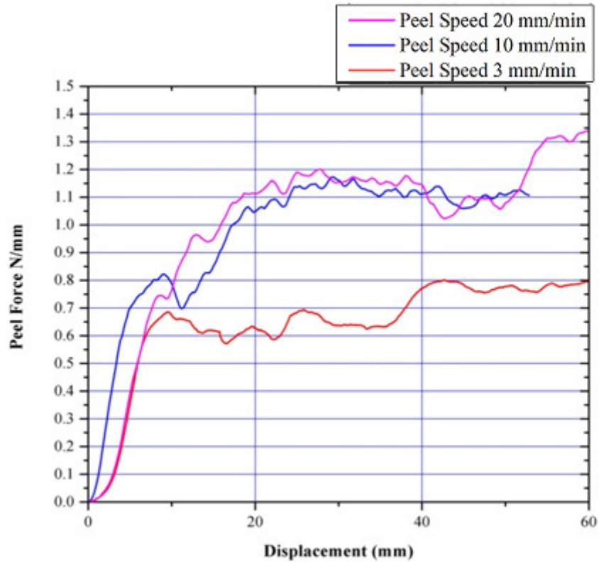
Figure 5.40. Experimental peel force for single-layer SMP – SS laminate at room temperature for different peel speeds.
