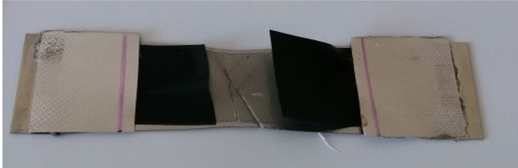
Figure 5.52. Delamination of SMP laminate of size 60 mm x 30 mm pre-strained to 35%, after 48 hours elapsed time following cutting.
