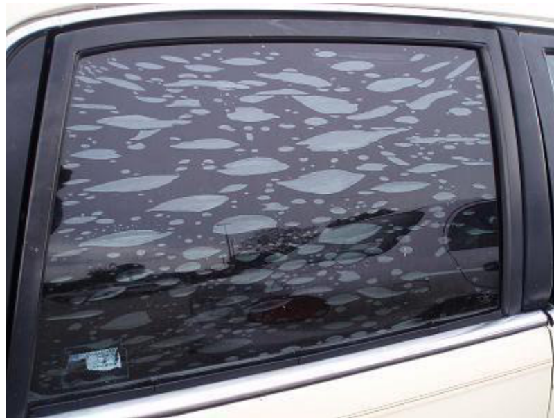
Figure 1.3. Wrinkles observed of car window tint as a result of weak adhesion between tint and glass [3].
