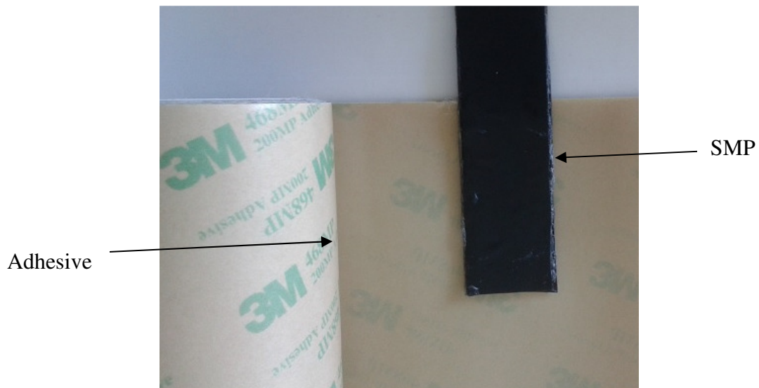
Figure 3.4. Process of applying adhesive to one side of SMP film.
