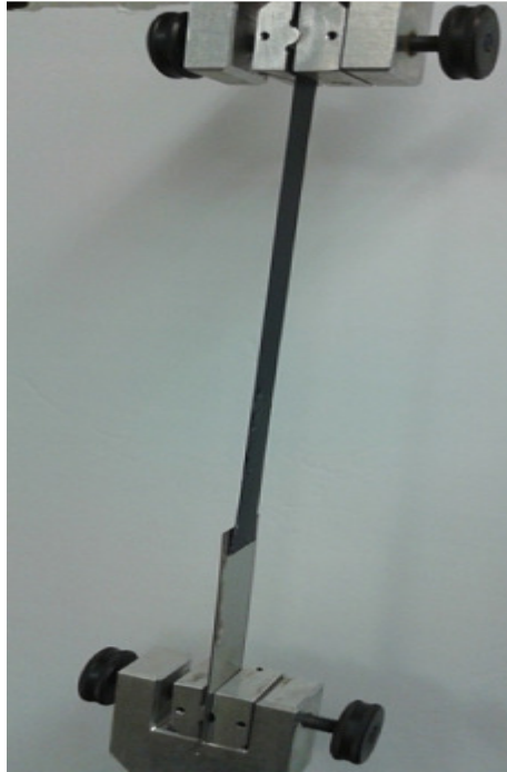
Figure 3.7. Photographs of 180° peel test specimens for 1-layer SMP-based laminate specimens showing large elongation of peel arm. Similar test with the 4-layer SMP-SS laminate significantly less elongation as noted in a later section.
