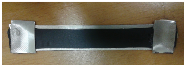
Figure 3.10. Laminate of size 80 mm x 20 mm after an applied engineering pre–strain of 35%.
