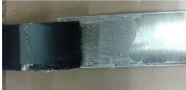
Figure 5.32. Four-layer SMP laminate specimen after peeling showing adhesive on the substrate (and not on the film), indicative of cohesive type of failure.
