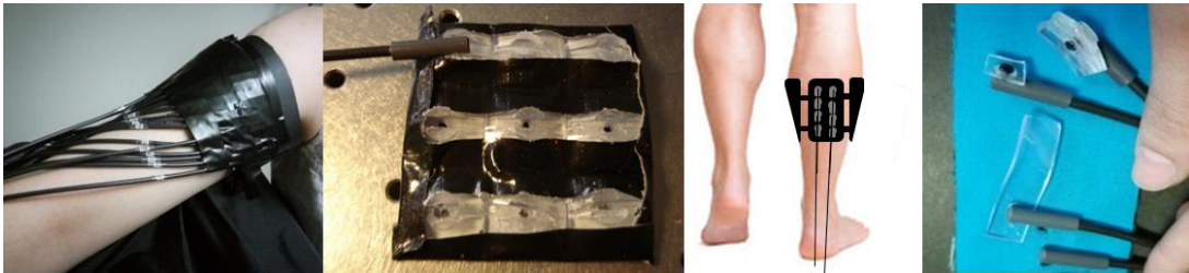
Figure 13. Concept ideas for in-vivo experimental measurements using the system's fiber bundle. Only non-magnetic materials were considered for this experiment and for future combined optical-MRI experiments with this system.
