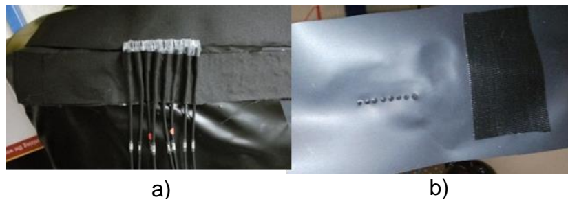
Figure 14. The probe holder designs made of a) suction cups and polyester (H1) and b) black silicone rubber (H2). Hole patterns were done using a hole puncher (H1) and a laser cutter (H2), respectively.
