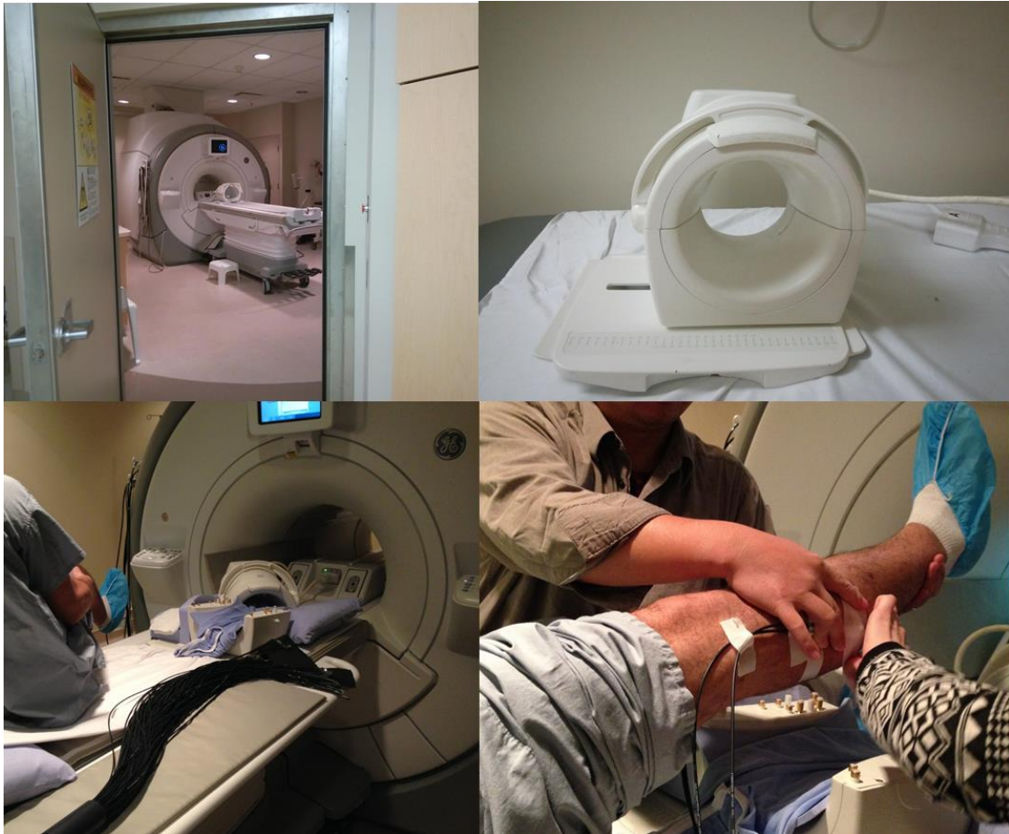
Figure 34. Photographs showing from the top-left to bottom right a) the MRI examination room, b) the MRI knee coil, c) the arrangement of the fiber bundle on the bed and d) the process of securing the measuring probes on the subject's leg.
