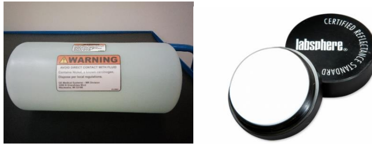
Figure 33. Photograph of the MRI leg phantom (left) and diffuse reflectance standard (right) to estimate the initial intensity delivered with the emitter probes. The measurements (total=20 images) were done along with a fragment of a BOLD-fMRI sequence to consider uniform experimental conditions. Emitter probes were secured on a diffuse reflectance standard using tape. The setup was then positioned on top of an MRI-leg coil to generate signal for the MRI and enable the sequence.
