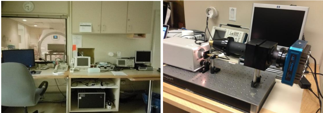
Figure 32. Photographs showing the configuration of the optical setup in the MRI control room. The photograph in the left shows the MRI control room and the one in the right includes the arrangement on the DOS system in the MRI control room.
