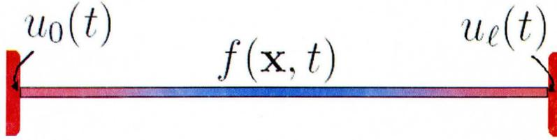
Figure 2.1: One-dimensional bar which is heated at both ends.
