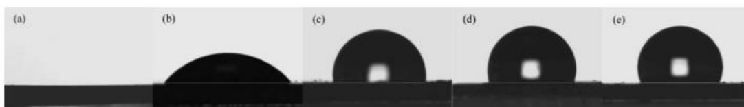
Figure 1-7: Water contact angles of various BaSO 4 nanoparticles modified with increasing concentration of ODP (Octadecyl dihydrogen phosphate) (Reprinted from Bala et al. [92] ).
