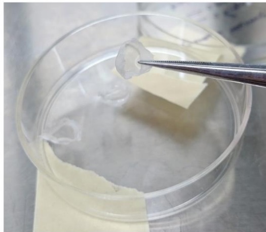
Figure A.3. PLGA and capsaicin-embedded PLGA discs were stored in sterile Petri dishes prior to being implanted in mice. Implants had a diameter of 1 cm and a thickness of 0.17 mm. Residual PLGA, seen on the outer edge of the disc, was not removed.
