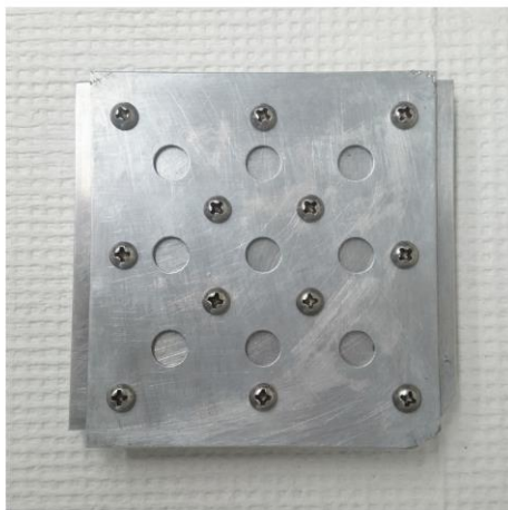
Figure A.4. (a) Stainless steel mold used to cast PDMS discs. Wells are 1 cm in diameter and 1 mm depth. (b) Discs were removed from the mold and autoclaved before undergoing PDA surface modification.
