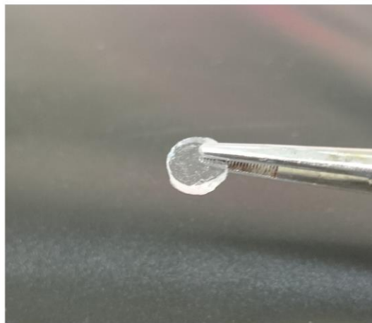
Figure A.4. (a) Stainless steel mold used to cast PDMS discs. Wells are 1 cm in diameter and 1 mm depth. (b) Discs were removed from the mold and autoclaved before undergoing PDA surface modification.
