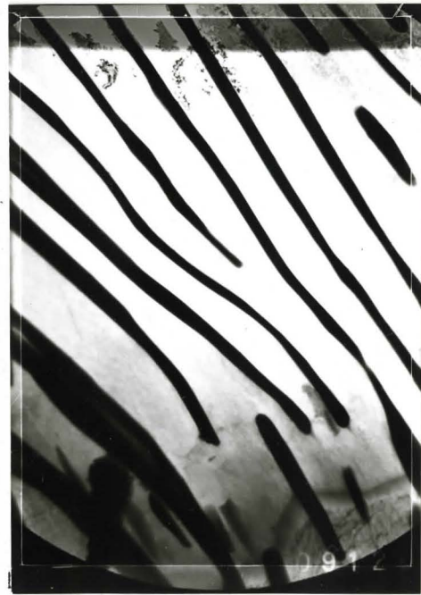
LG, Longitudinal section to tensile axis Fig. 9: A typical transmission electron micrograph of lamellar steel before the test.
