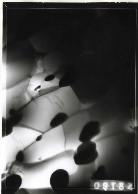
Fig. 14: Substructure of spheroidized steel showing no sub cell walls or dislocations in ferrite grains before the test.
