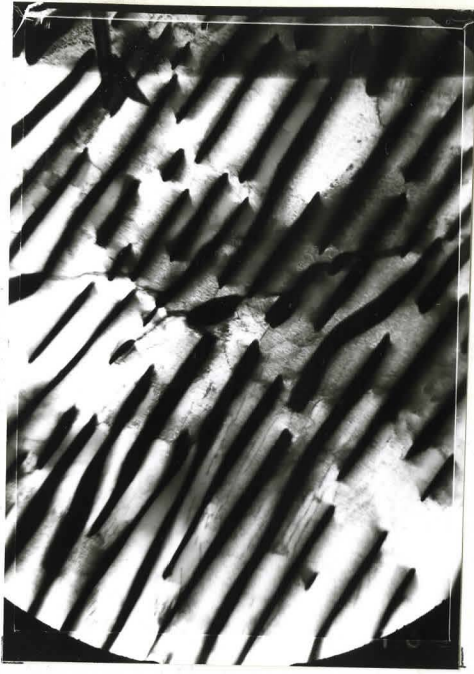
Fig. 12: Transmission electron micrograph of lamellar steel showing a grain boundary running across the lamellar structure.
