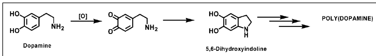
Figure 14 - Dopamine Polymerization. Dopamine polymerizes in aqueous alkaline conditions to form polydopamine. The exact mechanism is still debated. Adapted from [109].
