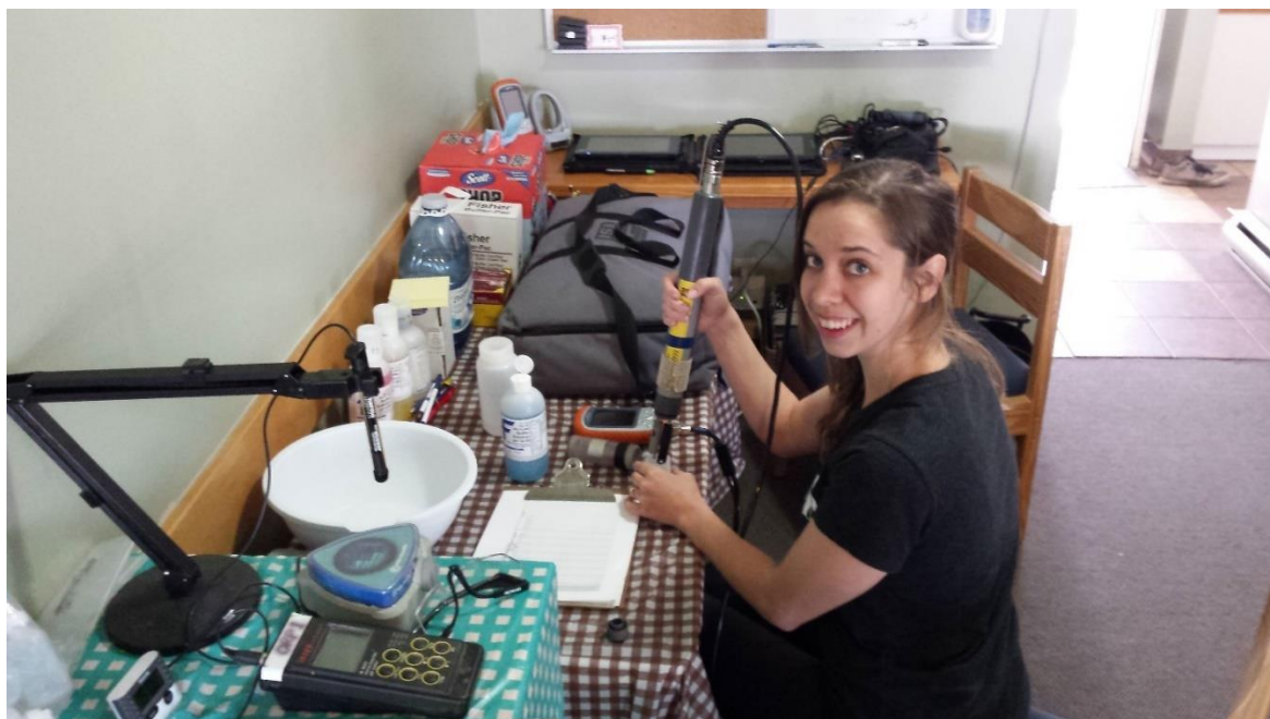
Figure 3.4: Morning calibration station for pH, Conductivity and Dissolved Oxygen.
