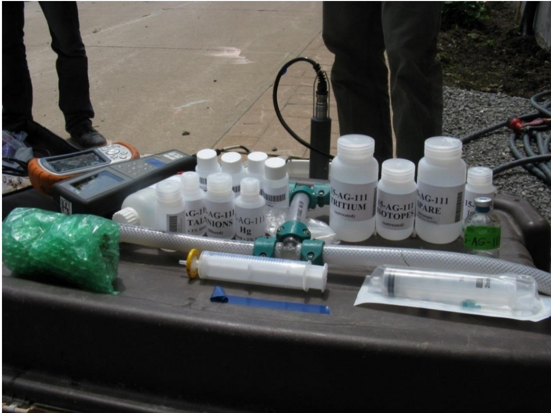
Figure 3.5: Sample bottles collected, field probes used and field filtration equipment at a field site.
