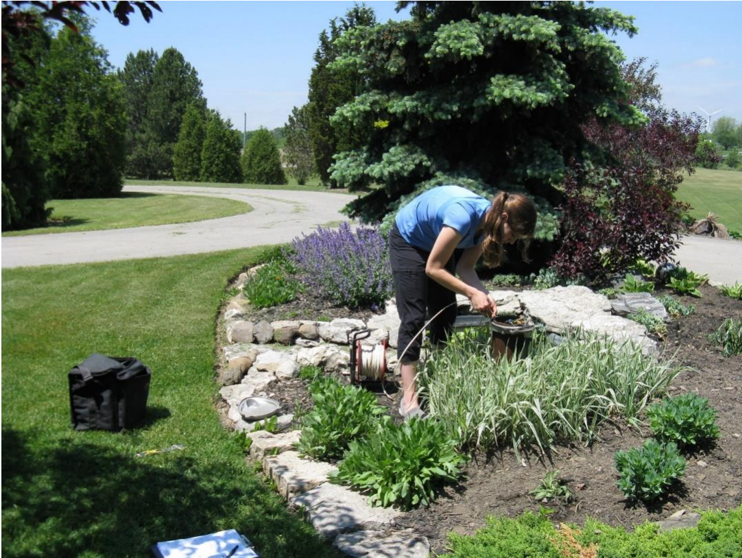
Figure 3.2: Obtaining static water level and depth measurements from a domestic well.
