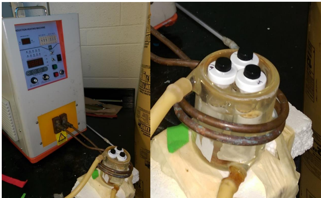
Figure S6.1: Photos of experimental AMF-activation assembly (left), with a close-up view of the Float-A-Lyzer devices in the jacketed flask within the device (right). The size of jacketed flask limited the number of Float-A-Lyzer membrane devices that could be used in a single experiment to three, so two separate experiments with two samples each had to be performed to achieve n = 4 replicates.
