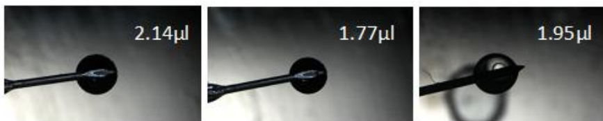
Figure 5.5: Example of small variation in droplet size from a 2 \mu\text{L} microinjection system developed from a mould generated using photolithography.
