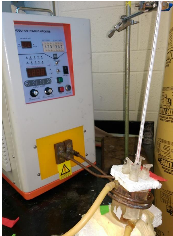
Figure S7.1: Picture of the AMF triggering apparatus. The nanocomposites are held in the test tubes by custom polyethylene holders and positioned at equivalent locations with the coils of the solenoid.
