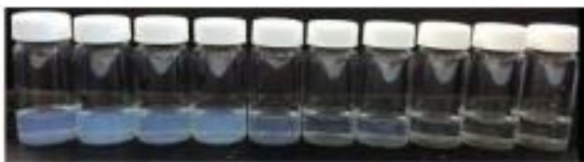
Figure 4.1.5 Images of nanogel formulations with varying contents of DMAEMA (remainder being DEGMA). From left to right: 0,20,30,35,40,45,50,60,80,100 (%DMAEMA). Images were taken of aliquots at room temperature after brief agitation.
