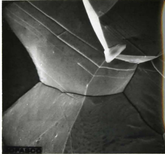
Figure 49. Scanning Electron Micrograph of NPL iron after 300 mins. illustrating surface markings on fracture surface. X500
