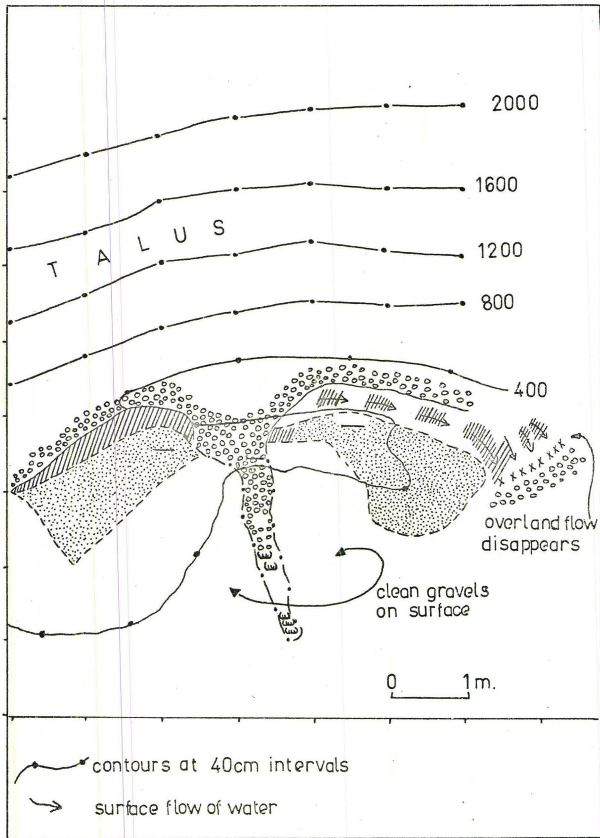
Fig. 6:I4 Distribution of fines at break of slope site B I97I.
