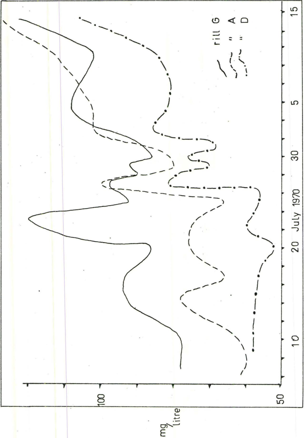
Fig. 4:7 Total hardness for rills A,D and G.
