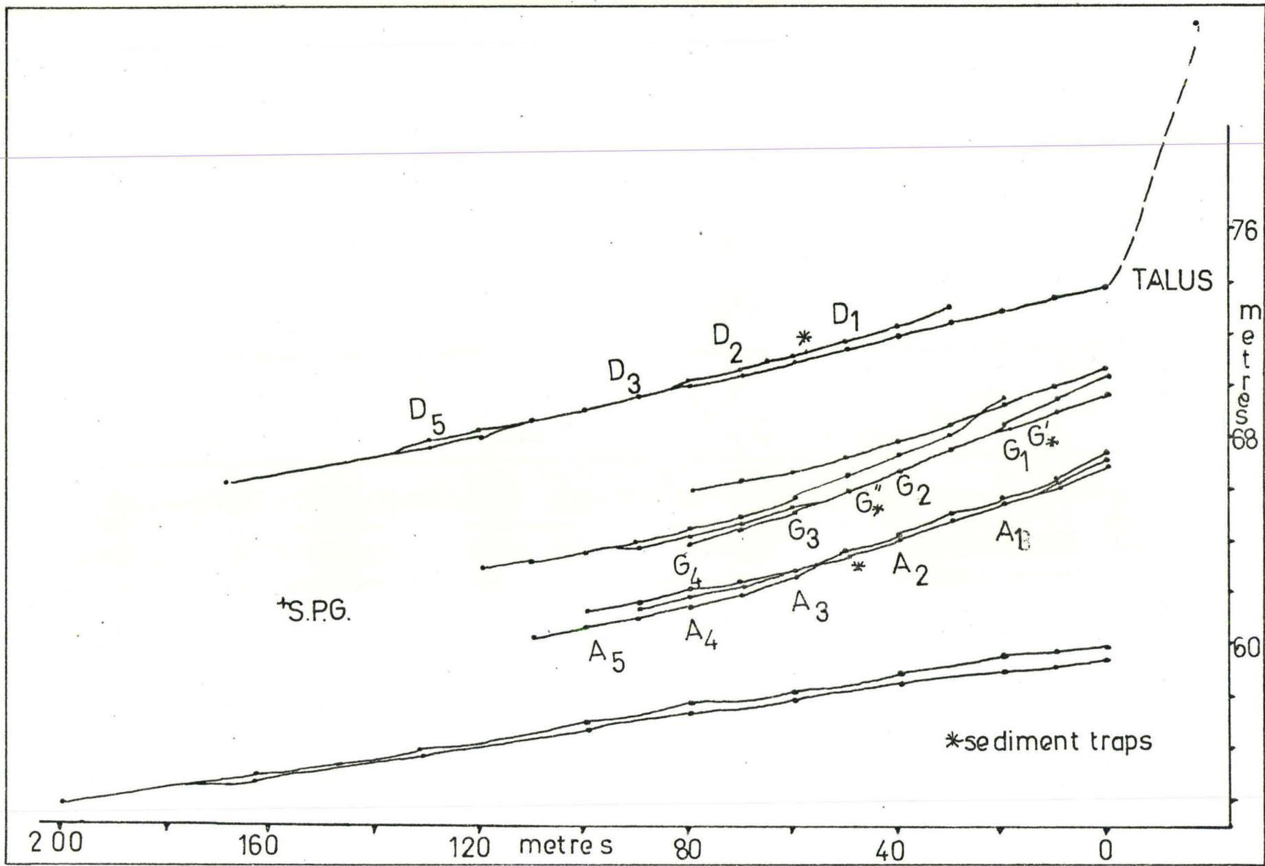
Fig. 2:6. Surveyed profiles of foot slopes.
