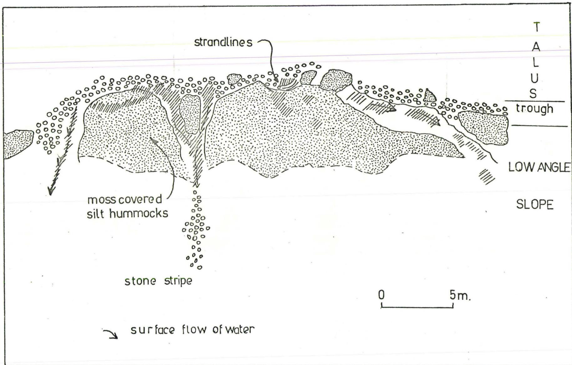
Fig. 6:15 Distributions of fines at break of slope near site B 1971.
