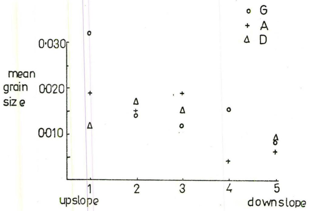
Fig. 6:7 Decrease in mean particle size down slope. Sample positions shown in Fig. 2:6.
