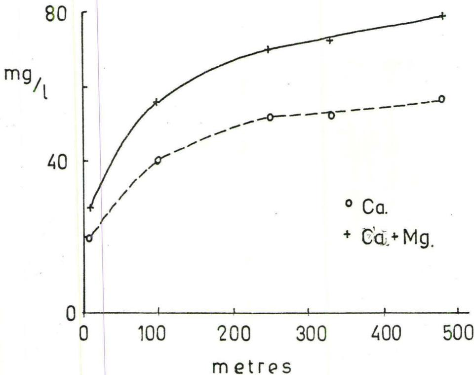
Fig 4:10 Increase in rill hardness values downslope on rill M 1971.
