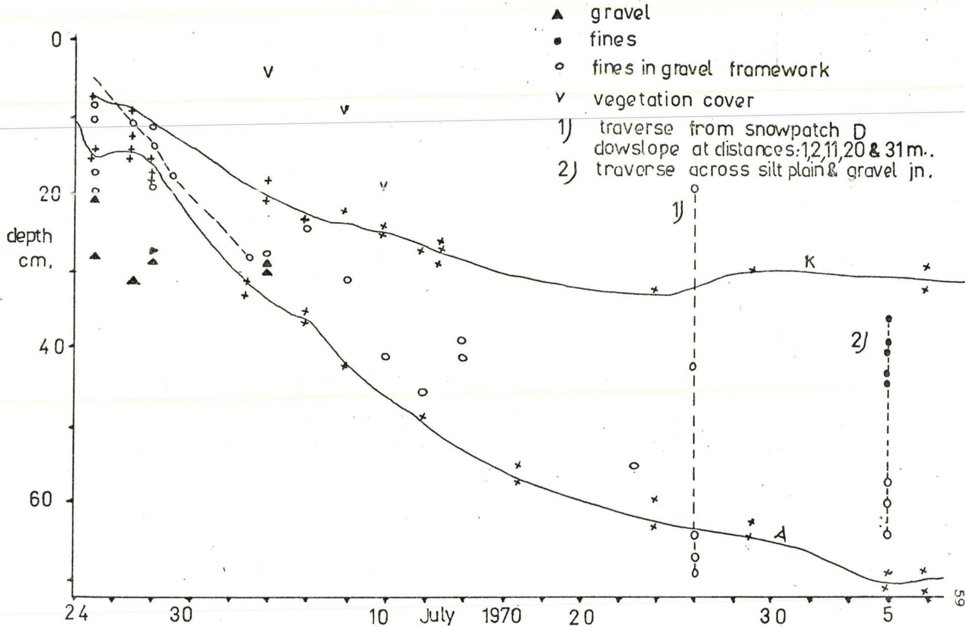
Fig. 4:3 Active layer thickness at various locations 1970.
