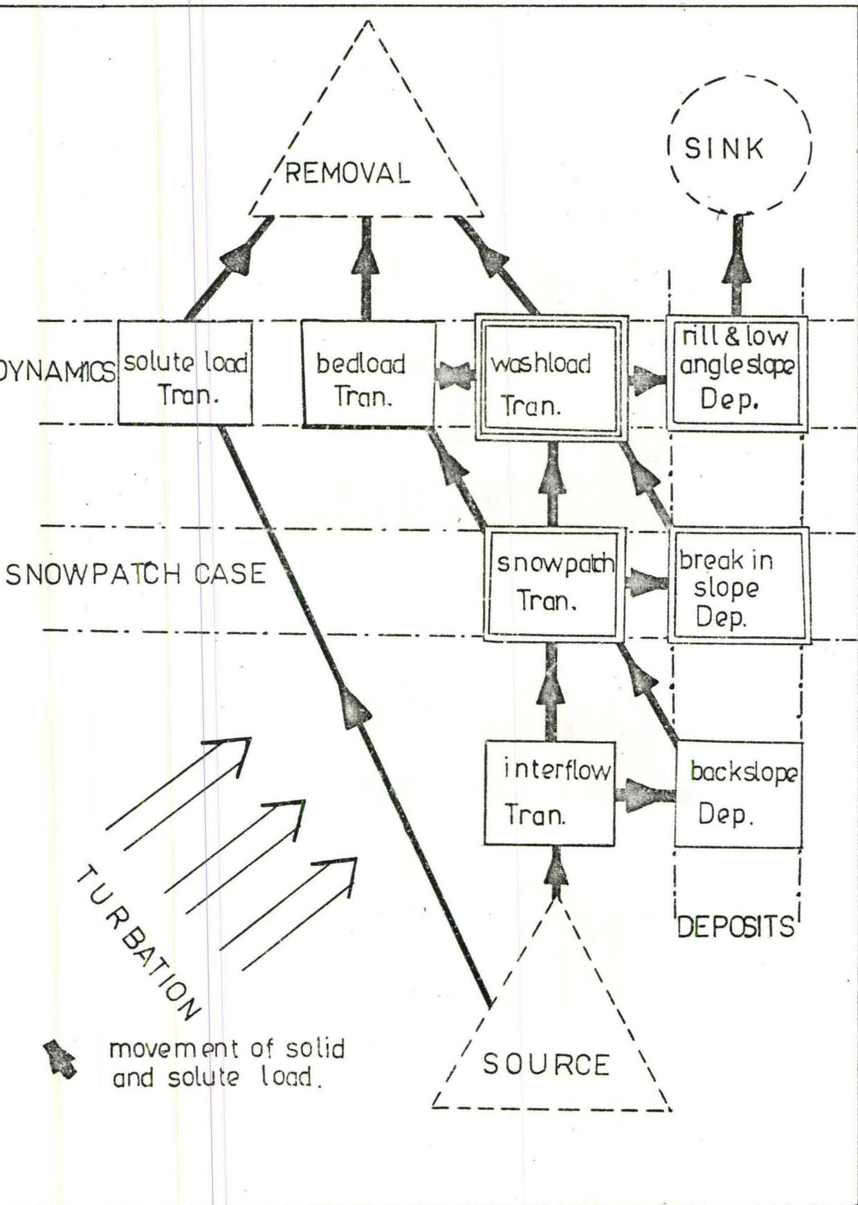
Fig. 7:1 Structure of the sediment transport system.
