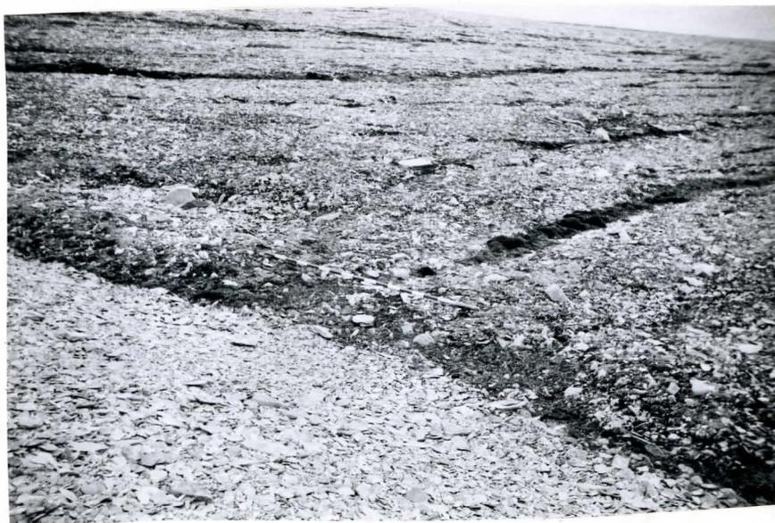
Fig 2:13 The interflow-overland flow junction, site D. Staff divided into 10cm. sections.
