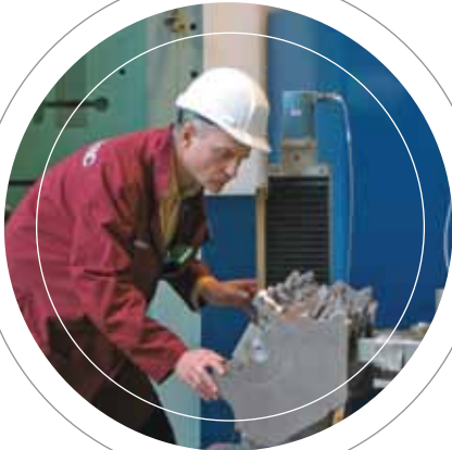
Studying the performance of aluminium in this prototype engine block for NemaK Inc.
