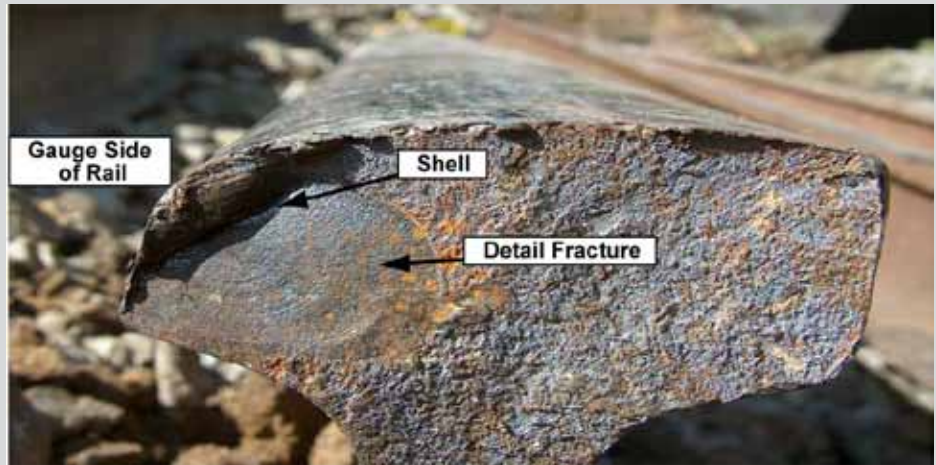
A fracture in rail recovered near Lake Wabamun, Alberta, after the derailment.
