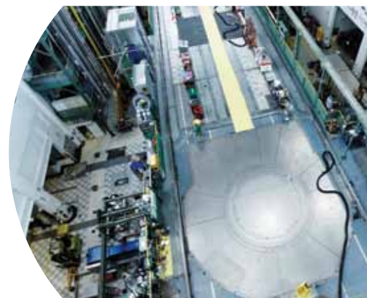
Top view of the National Research Universal (NRU) reactor, which supplies neutrons to the CNBC for materials research.
