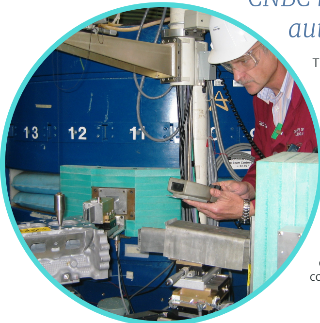
Dr. Dmitry Sediako prepares to measure stress in a GM cylinder head at the L3 neutron beamline.
