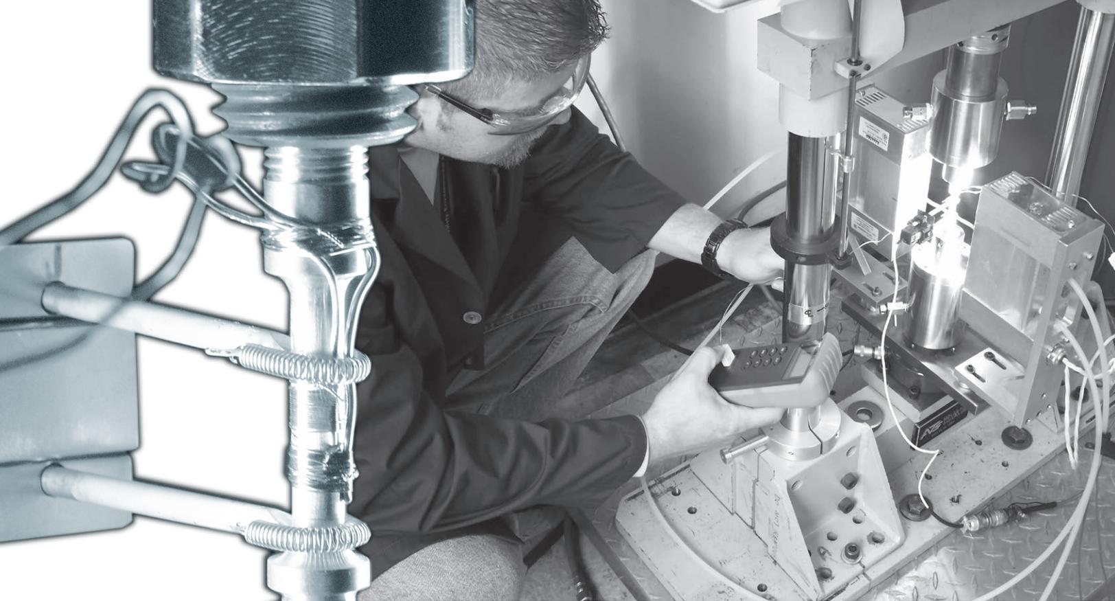
Labs and workshops adjacent to the guide hall are where more complex experiments are assembled prior to moving onto a neutron spectrometer. Pictured here, an industrial sample is mounted on equipment that will apply large forces, and high temperatures. Once on a spectrometer, neutron measurements will show scientists how the material responds to these conditions.
