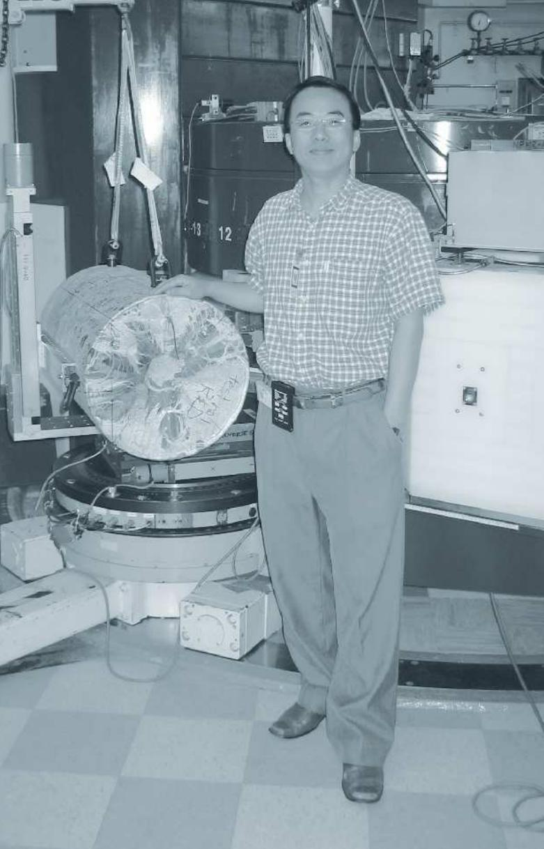
The ability of neutrons to penetrate materials enables researchers to probe the interior of large specimens (such as this magnesium casting, which is 50 cm in diameter and a meter long) and to acquire 3-dimensional maps of internal residual stress, non-destructively.
