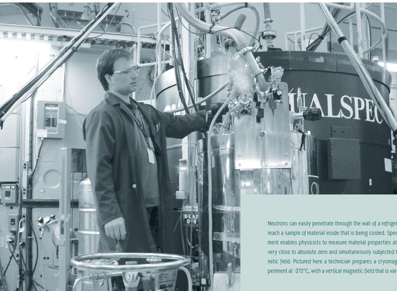
Neutrons can easily penetrate through the wall of a refrigeration unit and reach a sample of material inside that is being cooled. Specialized equipment enables physicists to measure material properties at temperatures very close to absolute zero and simultaneously subjected to a high magnetic field. Pictured here a technician prepares a cryomagnet for an experiment at  $-272^{\circ}\text{C}$ , with a vertical magnetic field that is variable up to 9T.
