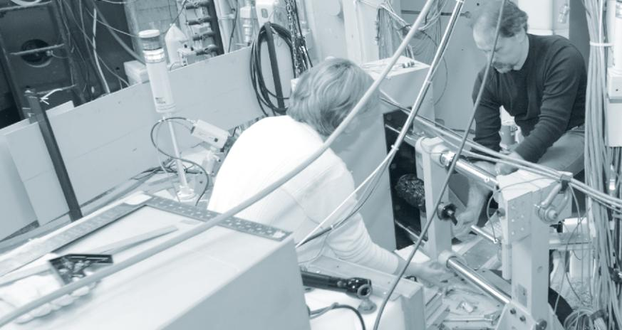
Neutron diffraction can reveal what is happening to the crystal structures (lattice distortion, texture evolution plastic damage, etc) of materials as they are subjected to loads and deformations. The loading instrument is installed directly onto the neutron diffractometer and its control is integrated into the main data acquisition system.
