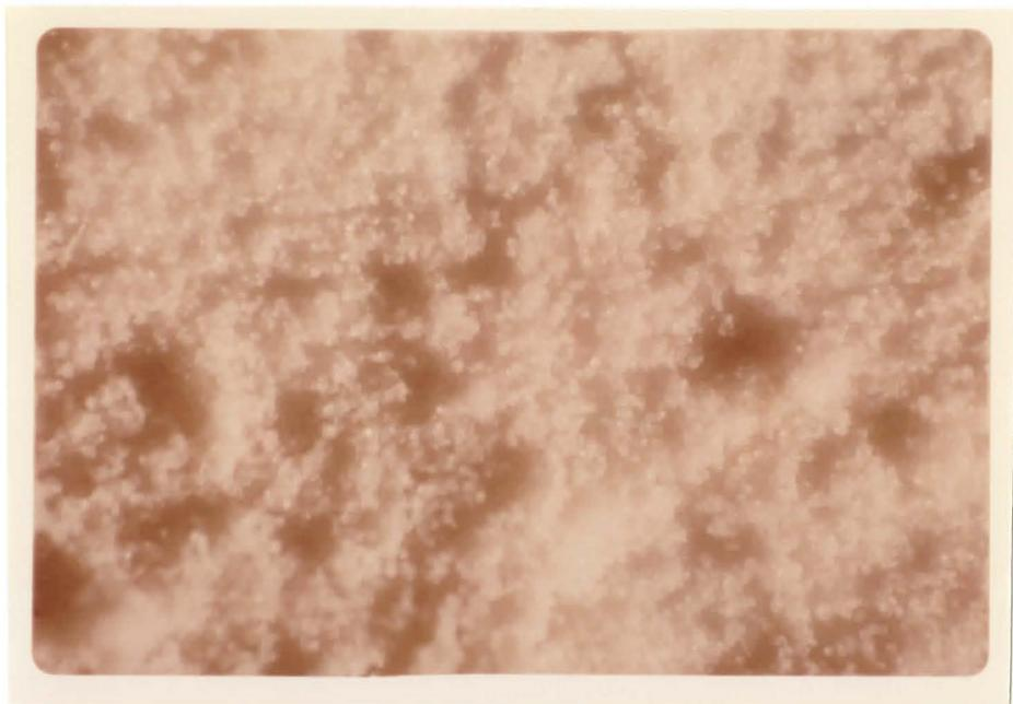
Fig. II.9.4. Pure product S. Crystals are spherical and somewhat transparent. They appear white when a number are present together. 1" = 0.535 mm.
