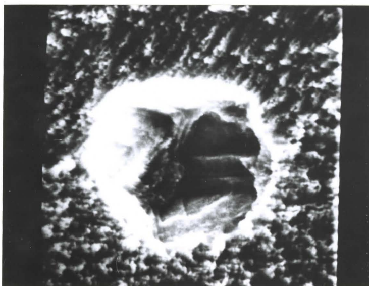
Figure 31. Morphology of pit formed on grain of \{100\} orientation with 40% cold work. 6600X. The exterior of the pit has become almost circular and no regular crystallographic facets exist in the pit interior. Pit size = 6.86 \mu .
