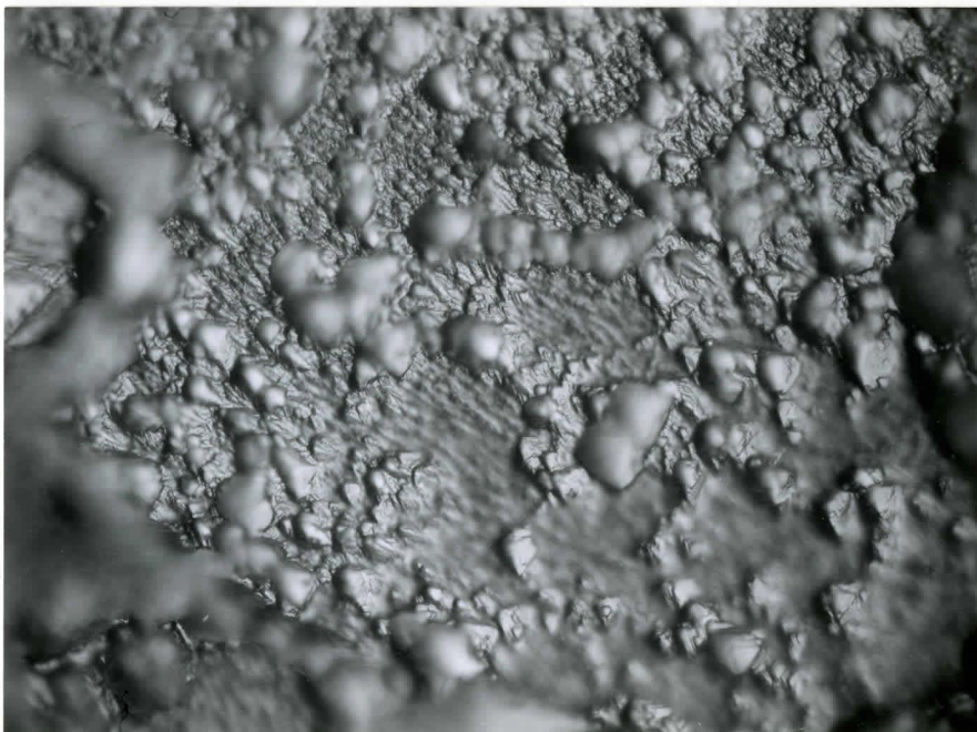
Figure 20(b). Magnified view of the grain interior attack. 620X. The appearance of the surface is typical of general corrosion.
