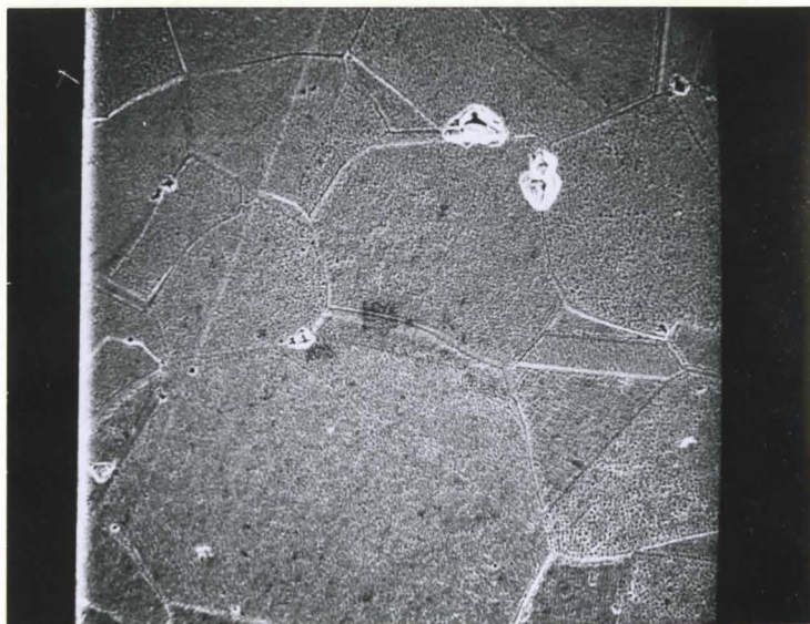
Figure 12. Pits at the grain boundary, 200X. Specimen G-3. Average grain dia. = 0.150 mm. Note that grain boundary grooving is absent.
