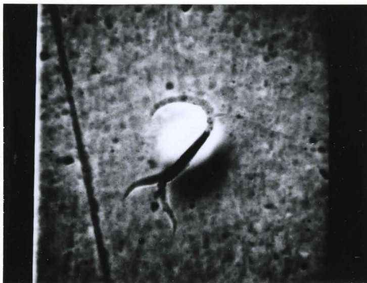
Figure 52. Development of pit in a 90% cold worked specimen. 5300X. Another pit in specimen of figure 51. Hump size - 3.0 \mu . The break has occurred across the hump. Very few such breaks were found.
