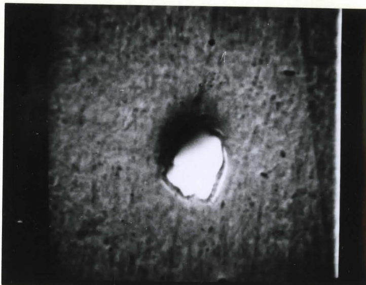
Figure 51. Development of pit in a 90% cold worked specimen. 5300X. Hump size - 3.0 \mu . The hump has broken at the edges. In most instances such breaks were found.
