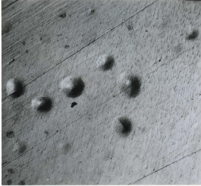
Figure 8(a). Surface of specimen of figure 7 after pitting corrosion. Un-etched. 80X
