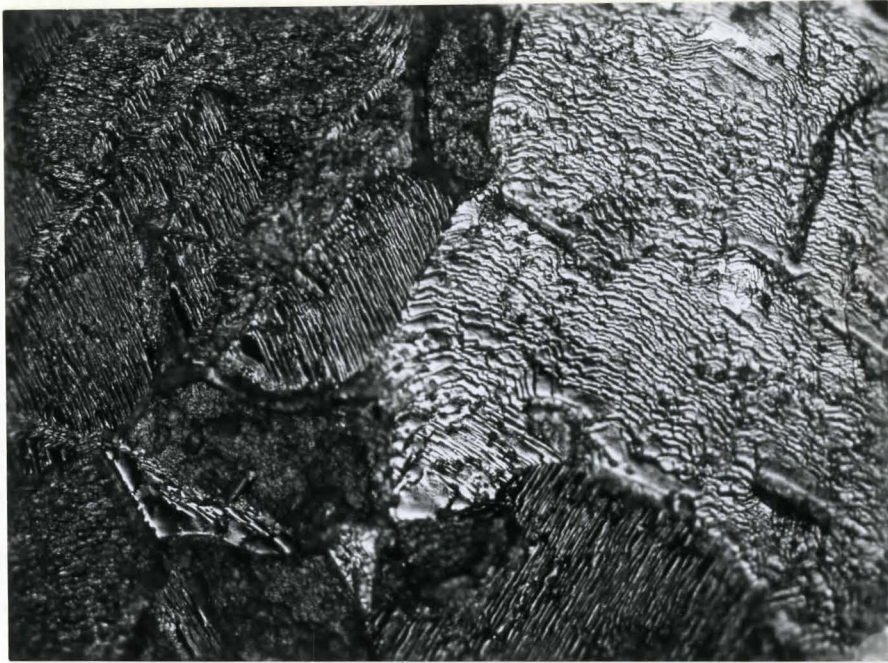
Figure 19(a). Surface of specimen A-2 polarized in 4 ml 1 N NaCl/100 ml 1 N H 2 SO 4 , 160X. Pits are still formed at the grain boundaries, but the attack spreads to the grains as well.
