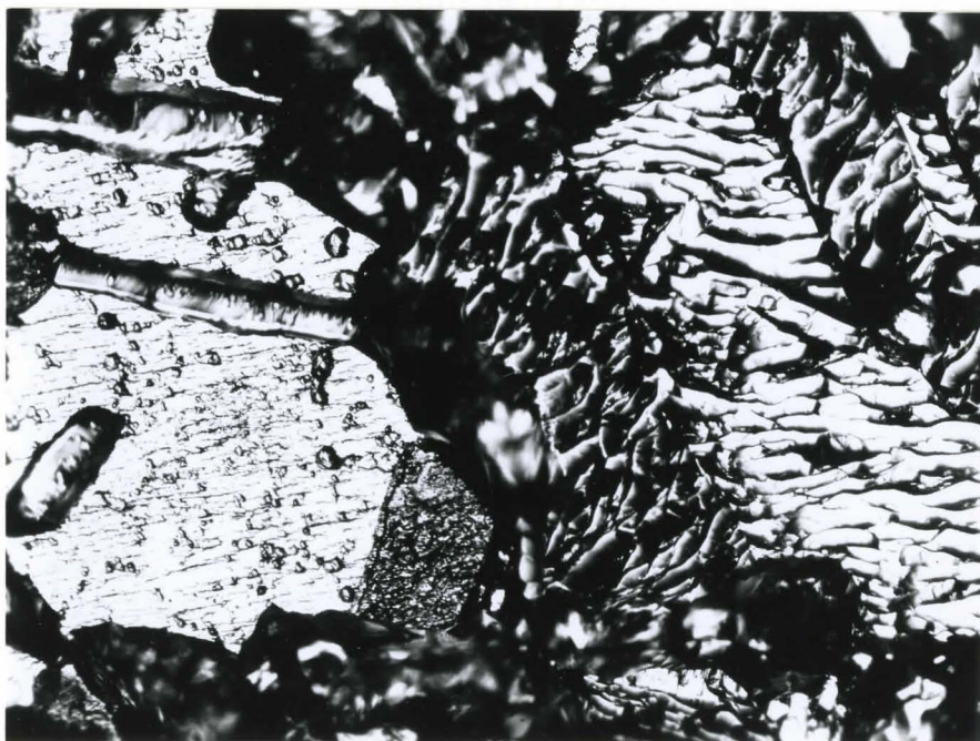
Figure 13. Attack on surface of specimen, 80X. Specimen G-4. Average grain dia. = 0.330 mm. Note that the attack is a mixture of general corrosion, pitting and deep grain boundary corrosion.
