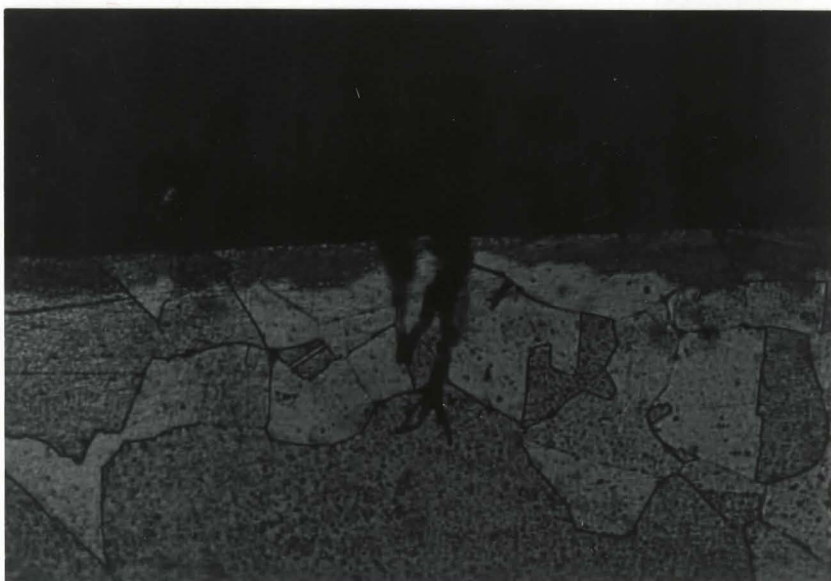
Figure 48. Grain boundary attack in an annealed specimen (dark field). 400X. The attack starts at the grain boundary but deeper into the material, becomes trans-granular. In this case, eventually a conical pit would have formed.
