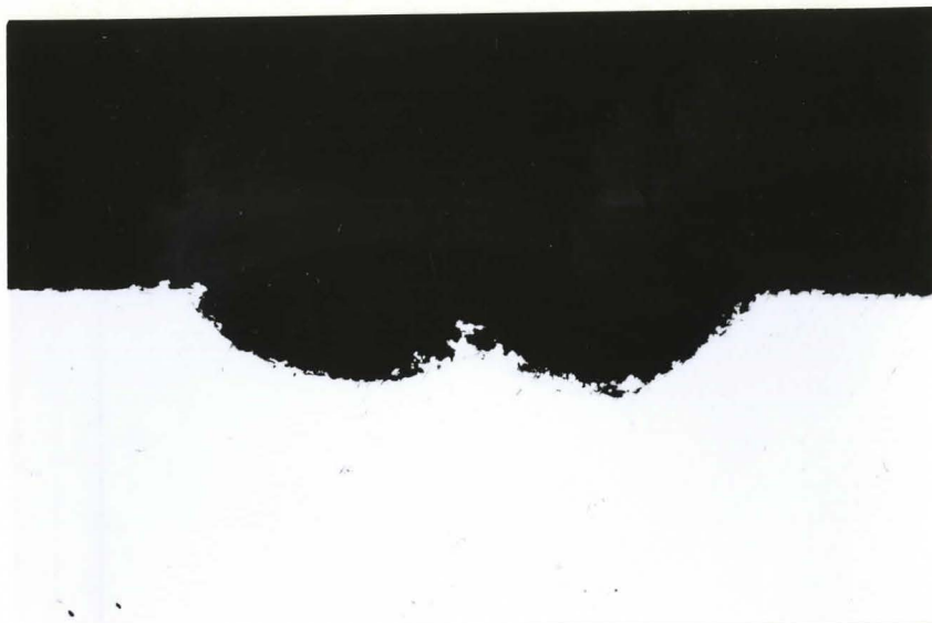
Figure 43(a). 'Saucer' pit (type 2) in a 90% cold worked specimen. Unetched. 80X. The pit is a combination of two shallow impressions.
