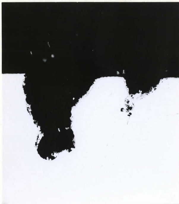
Figure 41. 'Conical' pits in a 90% cold worked specimen. 80X. The number of such pits was very small.
