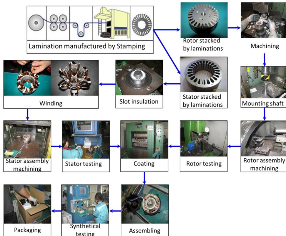
Fig. 2.10. Main manufacturing process of electric machines [77]. stator and rotor will be assembled together and some related tests will be done to make sure the electric machines are qualified.
