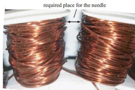
Fig. 2.20. Two needle-wound coils of the outer-rotor prototype motor [78].
