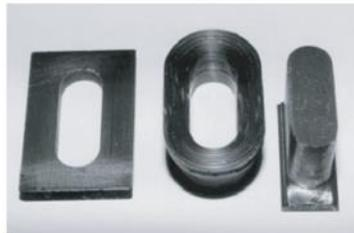
Fig. 2.15. Part of stator yoke, pre-pressed coil, and tooth in SMC from Jack [83].
