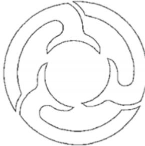
Fig. 2.14. Mecrow's segmented lamination for easy insertion of pre-wound coils [82]
