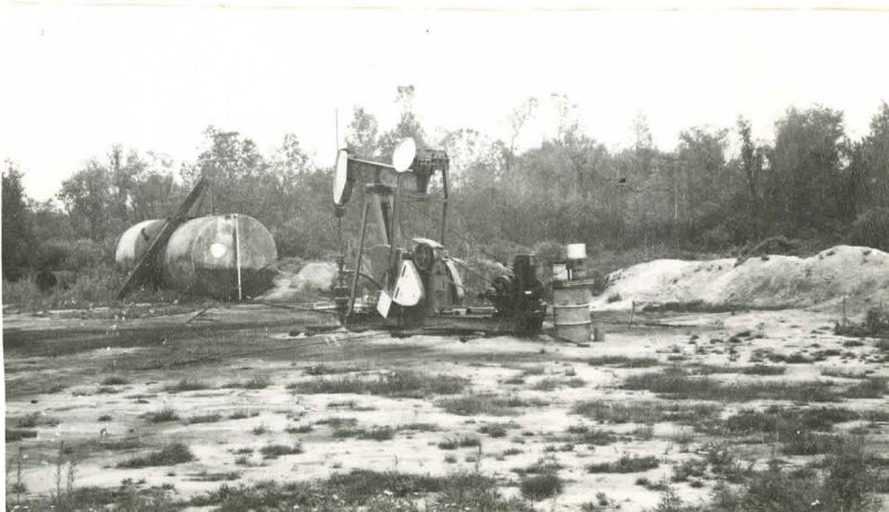
No. 56. The only oil well in Blandford is hidden on scrub land on the sand plain. Producing 6-8 barrels daily, it is an outlier of a small oilfield south-west of the township. Petroleum being of minor importance locally, it is not discussed in the text.
