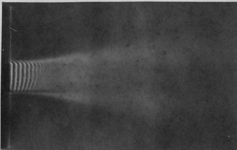
Flow from inlet nozzle (viewed along length of nozzle when tilted 15^{\circ} )
