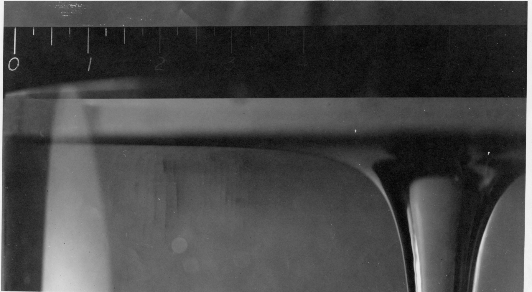
Fig. 15-Photograph of Water Vortex from Plexiglass Generator
