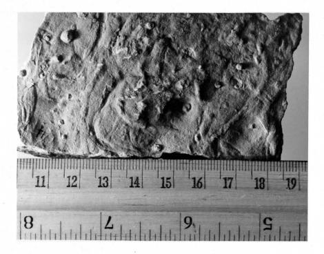
Plate 1: A typical sample slab of Thorold sandstone showing vertical worm tubes. If this specimen was larger, the number of strata that the outcrop would be divided into would be reduced.
