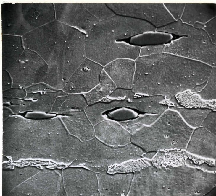
Fig. 2.6. Microstructure of AISI 12L15 Steel in Longitudinal Direction.
