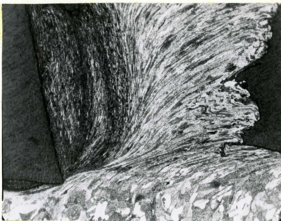
Fig. 3.30 Metallographic Specimen Resulting from Quick Stop Device at the Cutting Speed of 55 ft/min. for AISI 1018 Steel.
