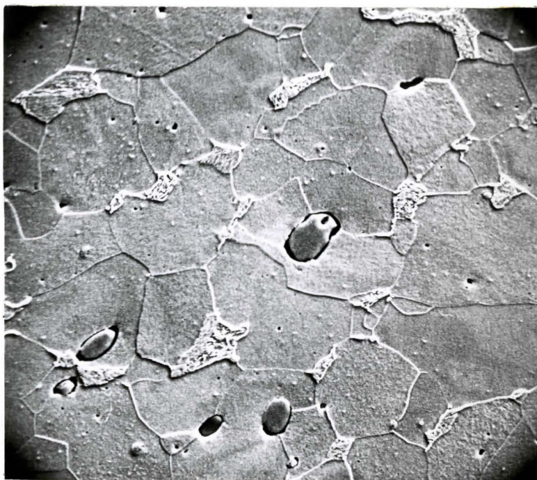
Fig. 2.5. Microstructure of AISI 1215 Steel in the Transverse Direction
