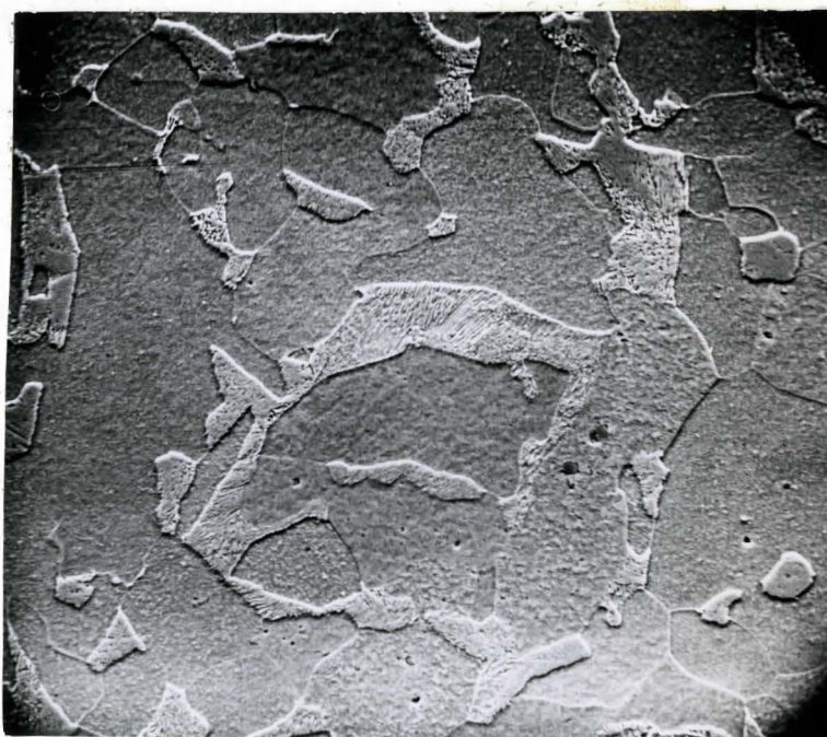
Fig. 2.3. Microstructure of AISI 1018 Steel in the Transverse Direction
