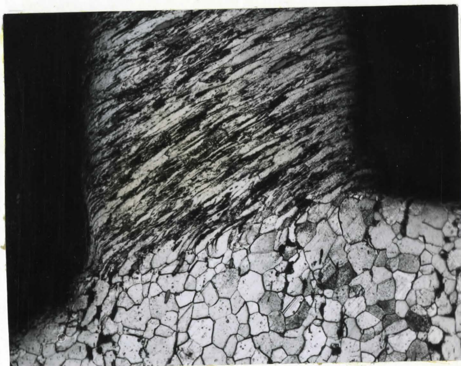
Fig. 3.28. Metallographic Specimen Resulting from Quick Stop Device at the Cutting Speed of 200 ft/min for 1215 Steel.
