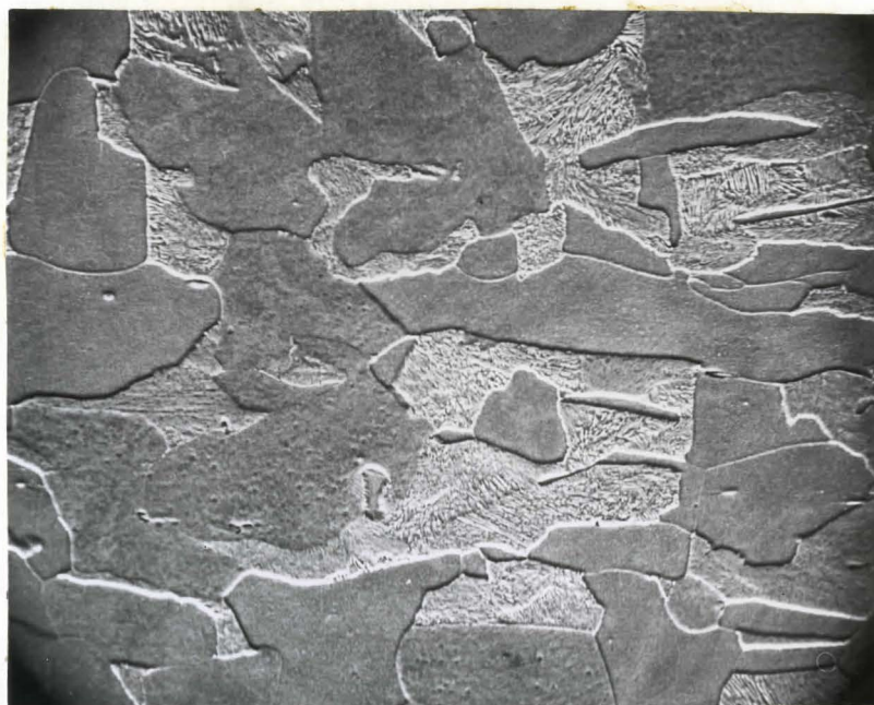
Fig. 2.2. Microstructure of AISI 1018 Steel in the Longitudinal Direction.
