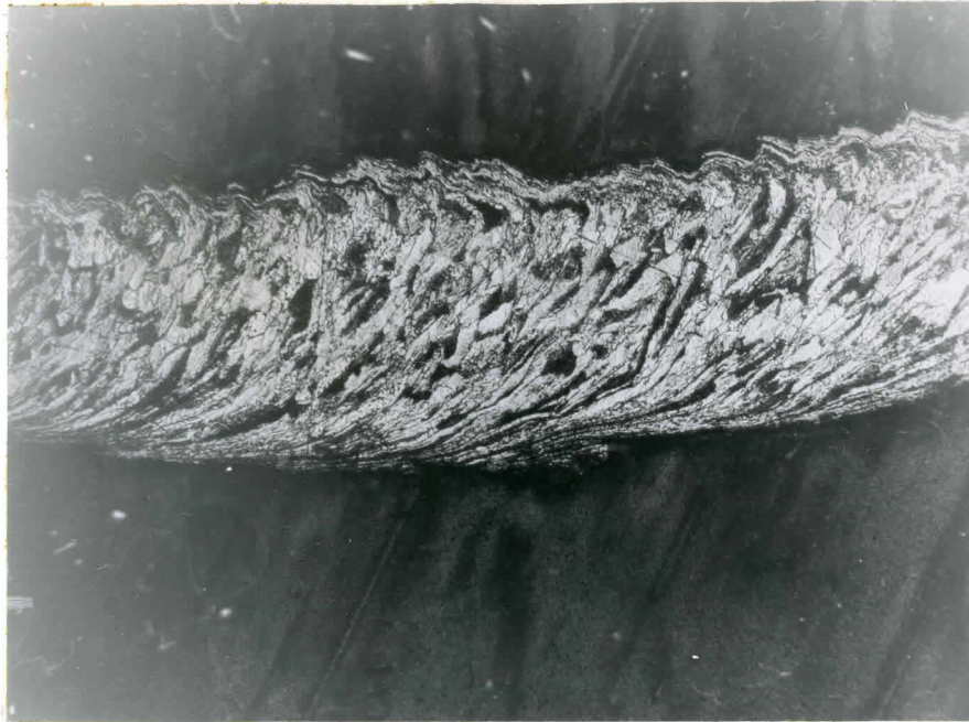
Fig. 4.2. Chip Photomicrograph of AISI 1018 Steel at the Cutting Speed of 100 ft/min.
