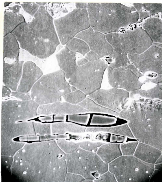
Fig. 2.4. Microstructure of AISI 1215 Steel in the Longitudinal Direction.
