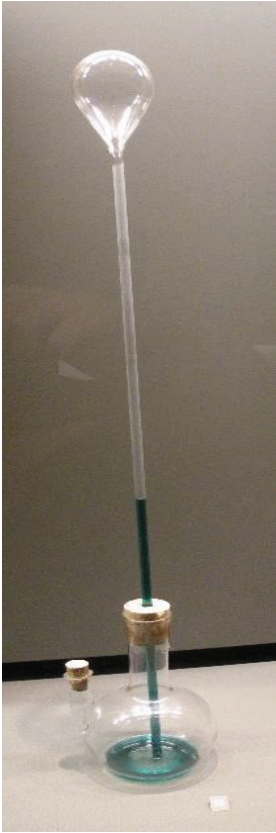
Figure 3.27: The thermoscope depicted contains a coloured liquid to allow for ease of observation. As the temperature of the system decreases the air within the bulbous section of the instrument contracts and the liquid rises. As the temperature of the system increases the air expands and the fluid lowers. These pre-thermometers were useful at examining changes in temperature but not actual values of thermal energy.
