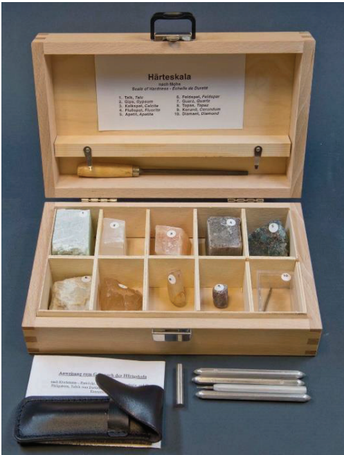
Figure 3.21: A typical kit containing Mohs' ten minerals, often used for scratch tests in the field
