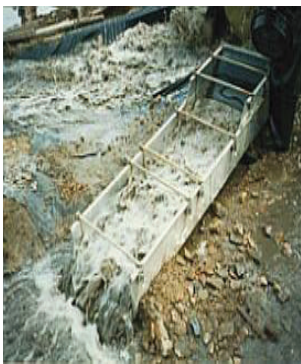
Figure 4.6.8: A placer mining sluice box, similar to those used in gold washing throughout ancient Egyptian history.
