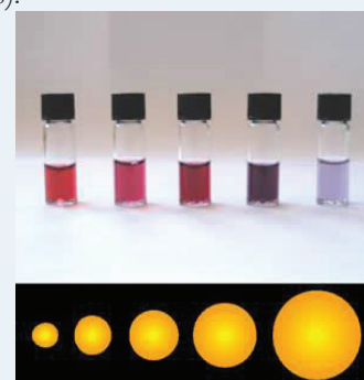
Figure 4.6.9: Various gold nanoparticle solutions. The colour of each solution is dependent on the size of the particles within. This property is linked to gold's optically reflective interactions that dictate the nanoparticles reaction to electromagnetic radiation, such as RF radiation.
