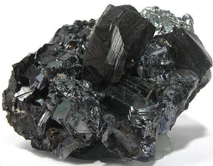
Figure 4.1.3: A sample of sphalerite and galena from the F. John Barlow collection. sphalerite, the dark black mineral with a non-metallic or submetallic lustre, is often associated with galena, the mineral with a metallic lustre.
