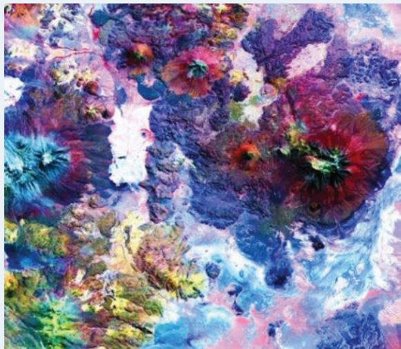
Figure 3.8.4: An ASTER image of the Andes. ASTER images can be used to monitor the volcanic activity in a region. The colour of the fringes indicates areas of surface deformation and the rate of movement of the ground. Patterns of multi-coloured swirling are indicative of areas undergoing the most surface deformation.
