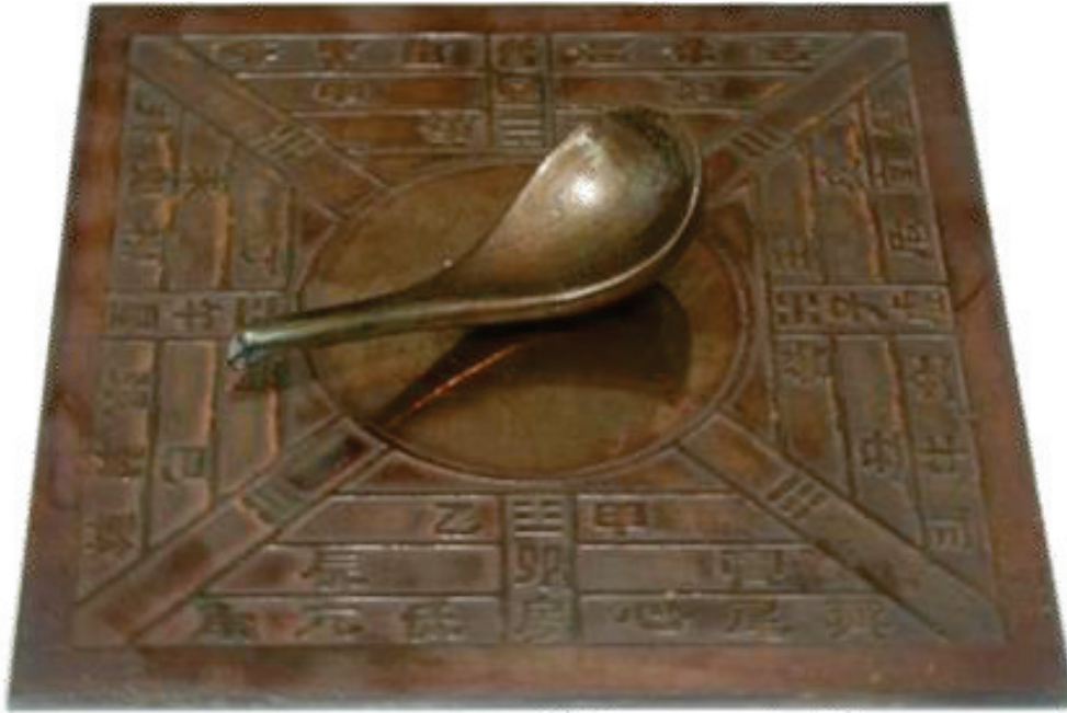
Figure 3.3.2: The earliest known design for a Han Dynasty (206 BC – 220 CE) South-Pointer. A spoon-shaped lodestone placed on a square brass plate with a circle at its center.
