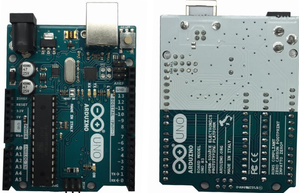
Figure 5: Arduino Uno R3 programmable circuit board (PCB). This is the board onto which the entire operating sequence is loaded, and which controls the incubator's behaviour.
