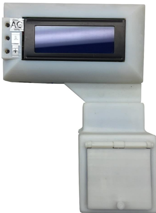
Figure 13: Final, assembled version of the second generation of the incubator. Note the programmable core of the incubator to the left of the photo with the LCD display on top. This programmable unit can be programmed to interface with a wide range of attachments, thereby greatly increasing the potential function of this device. The final incubator is suited to programmable temperature profiles, steps, holds and stages. Final input voltage accepted ranges from 8V – 15V, or USB.
