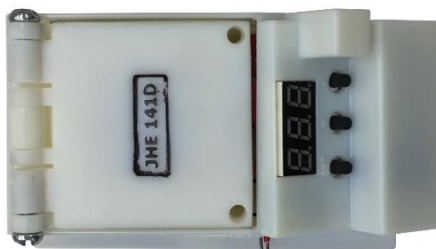
Figure 12: Final, assembled version of the first generation of the incubator. Note that this is solely an isothermal incubator, not suited to adaptable temperature profiles or different functions. Final voltage input ranges from 9V – 12V.
