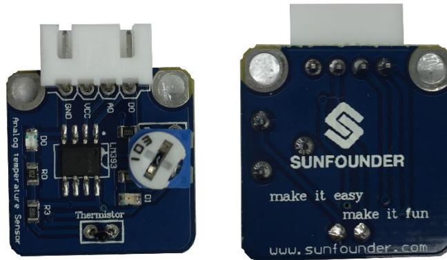
Figure 9: Sunfounder thermistor and amplifier set for Arduino. Temperature sensitivity is \pm 0.01^{\circ}\text{C} , and is delivered to the Arduino to modulate temperature and display on the LCD.
