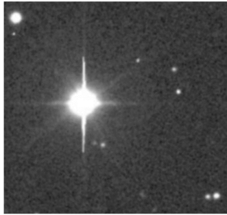
Figure 1.9: Blooming on a CCD image: the saturated vertical columns are the bloom. The other linear spikes on the bright star image result from diffraction by the vanes supporting the telescope's secondary mirror (Chromey, 2010).
