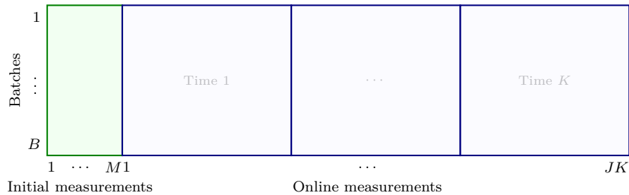
Figure 2.4: Rearrangement of the batch data in Figure 2.3 to form the regressor matrix for identifying the quality model in Equation 2.2
