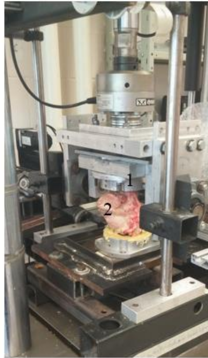
Figure 3.7: Anterior view of a fully mounted specimen, including dental plaster, placed in the Instron for loading where: 1) femur and 2) patella. The femur is placed superiorly to the tibia such that the top cup holds the femur.
