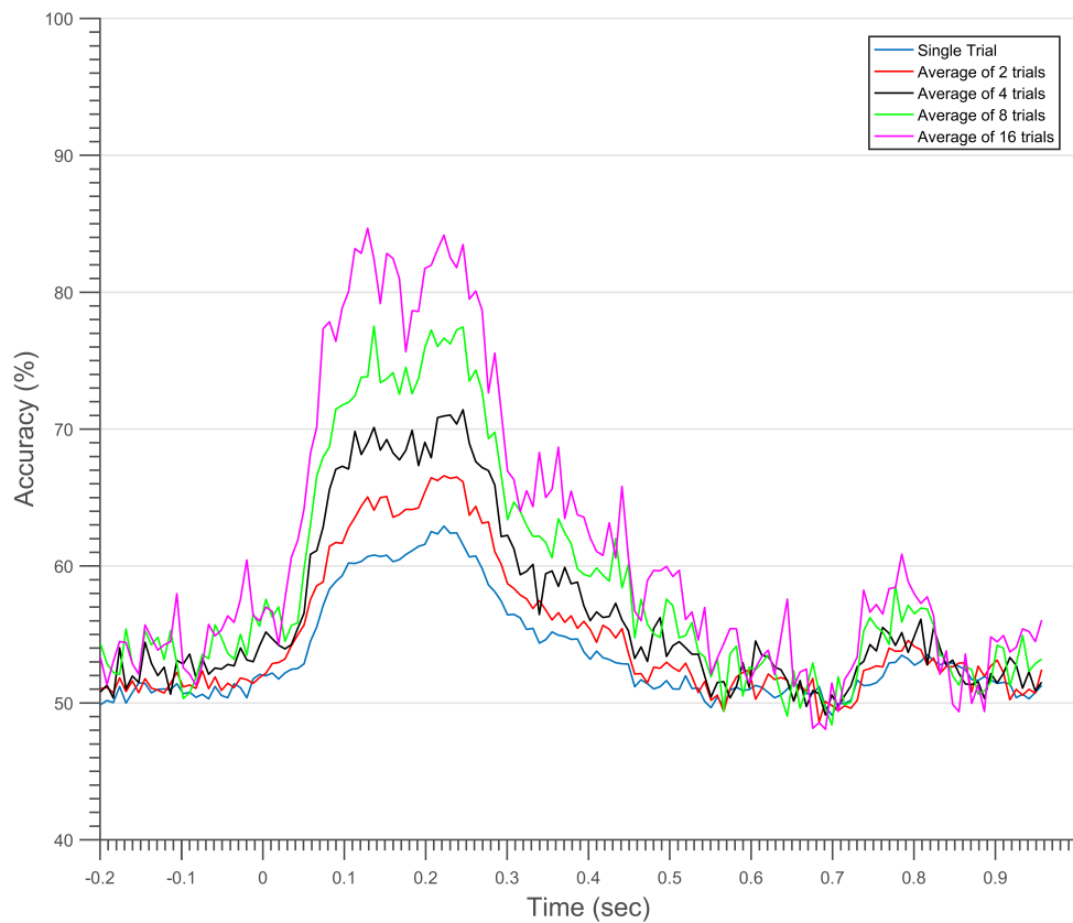
Figure 3.14: The accuracy of correctly classifying a frequency deviant from a standard tone trial in the MMN dataset using the proposed methods and showing the differences across the 5 different averaging settings.
