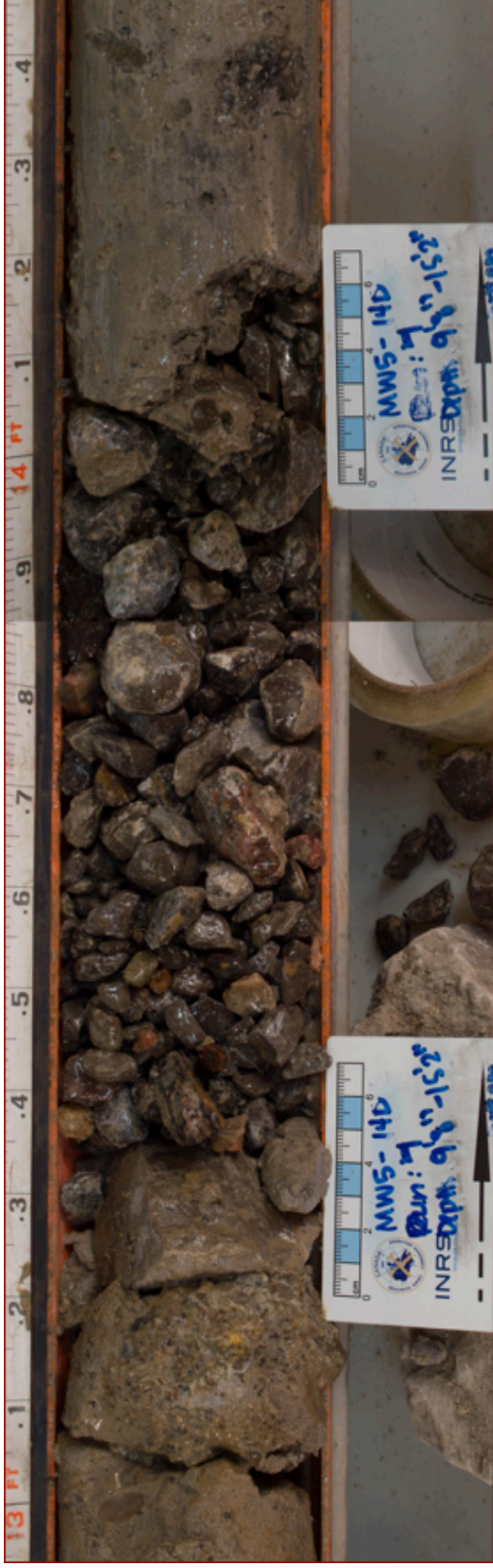
Figure 15: A washed out section of core approximately 33.5 cm in length located within the uppermost diamicton unit (Newmarket Till). This core section is located 2.99 – 4.63 m bgs.
