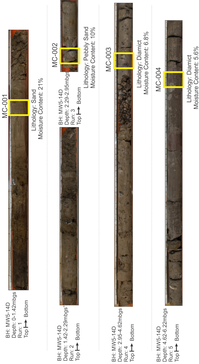
Figure 20: Lithological descriptions and results of moisture content (MC) by mass accompany sample locations (MC-#) in the first five core runs. The moisture content of the diamict units are below 10%, which is consistent with Newmarket Till (Sharpe and Russell, 2016). Note: the static water levels in the shallow water table well, MW5-14S(2), is 2.82 m bgs, therefore it is assumed that the diamict samples are saturated samples.
