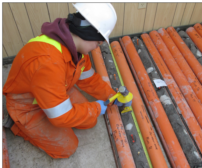
Figure 14: Obtaining grain size samples from the Newmarket Till required a hammer and wedge because the core material was over-consolidated and cemented.
