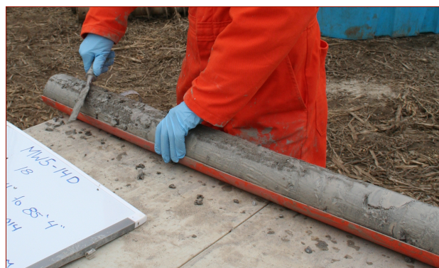
Figure 9: Drilling fluid coats the sediment core. Scraping tools are used to remove the film.
