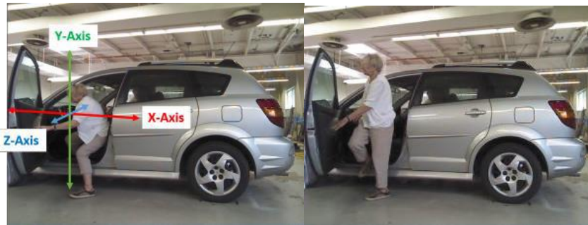
Figure 1-11. Still frames exemplifying the one-foot parallel egress strategy. The left frame illustrates the participant exiting the cabin while facing the front of the vehicle. The right frame illustrates the participant bringing her right leg out while standing on her left leg and facing the front of the vehicle.
