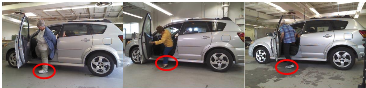
Figure 1-2. Still frames exemplifying the one-foot ingress sub-strategies: lateral sliding (on left), backward motion strategy (centre), and forward motion strategy (on right).
