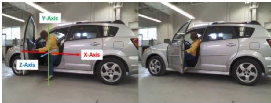
Figure 1-4. Still frame exemplifying a one-foot lateral sliding ingress strategy. The left frame illustrates the participant entering the cabin with her face parallel to the vehicle along the x-axis (i.e., looking forward at the vehicle hood while moving laterally along the z-axis into the vehicle cabin). The right frame illustrates the last stage of the ingress strategy where the participant flexes her hip and adducts her left leg inside the vehicle cabin.
