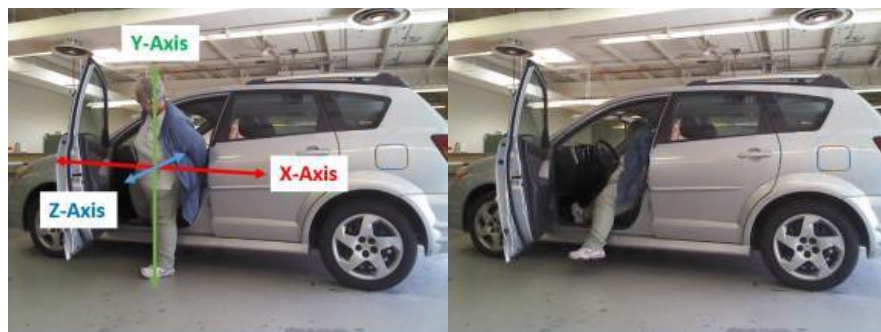
Figure 1-5. Still frames exemplifying a one-foot backward motion ingress strategy. The left frame illustrates the participant entering the cabin with her back facing the vehicle cabin along the z-axis. The right frame shows the rotation of the body after the participant sat down as she brought her left leg inside the cabin.
