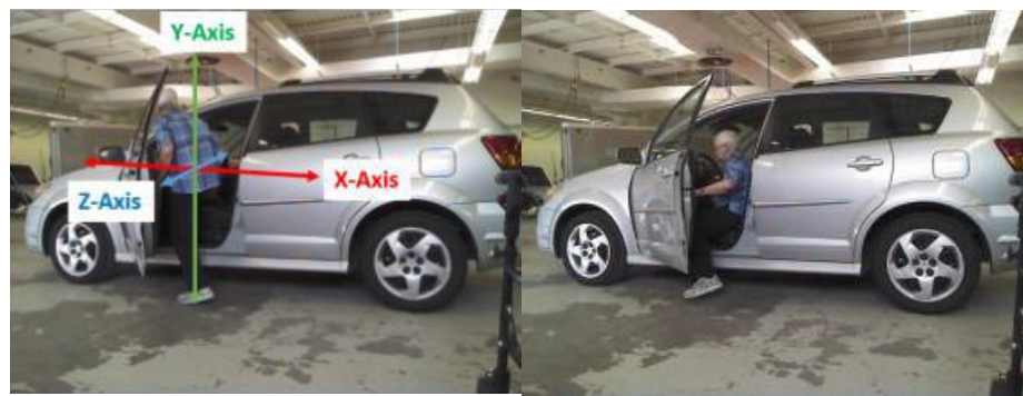
Figure 1-6. Still frame exemplifying a one-foot forward motion ingress strategy. The left frame shows the participant entering the cabin as her torso faces the interior of the vehicle cabin along the z-axis. The right frame demonstrates the rotation of the body as she brings her left leg inside the cabin while positioned in the seat.
