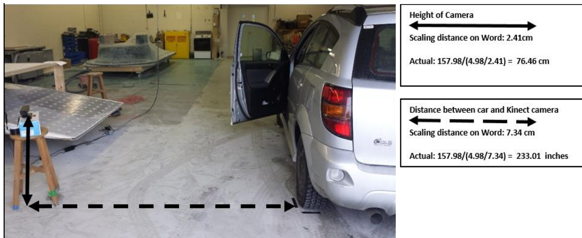
Figure 2-3. Positioning of Microsoft Xbox Kinect camera relative to the Pontiac Vibe. Note positioning of rear tire within the designated tape markings to ensure consistency across participants.
