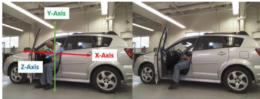
Figure 1-7. Still frames exhibit a two-foot trunk forward motion ingress strategy. The left frame illustrates the participant entering the cabin with both feet planted on the ground parallel to the vehicle. The right frame shows the participant bringing his left leg into the cabin once seated.
