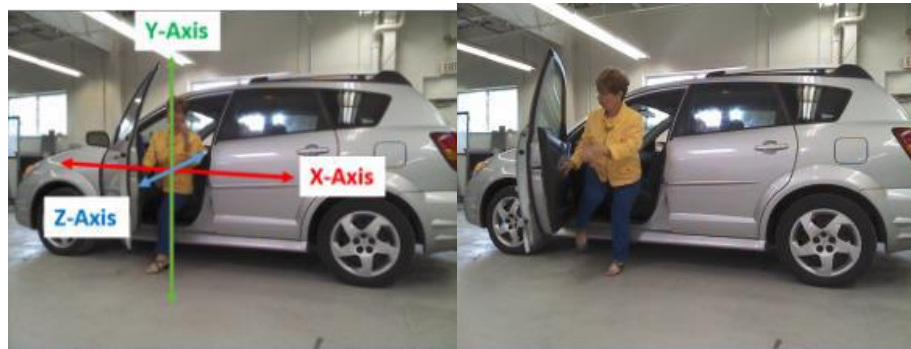
Figure 1-10. Still frames exemplifying the one-foot head forward egress strategy. The left frame illustrates the participant exiting the cabin while facing perpendicular (along the z-axis) to the orientation of the vehicle. The right frame illustrates egress, as the participant brings her right leg out of the cabin while standing on her left leg.
