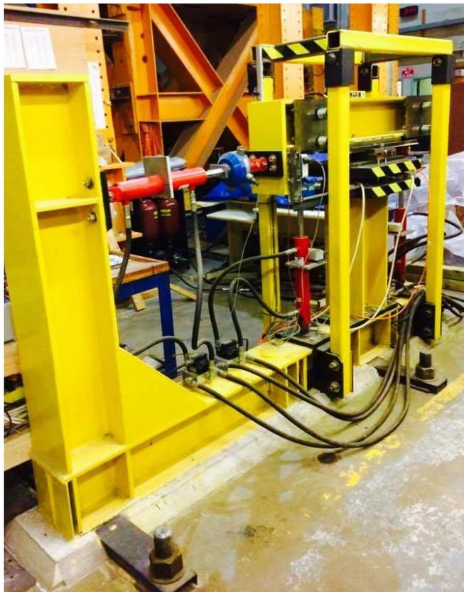
**Fig. 5-5:** Photograph of the three-degree of freedom test apparatus.
