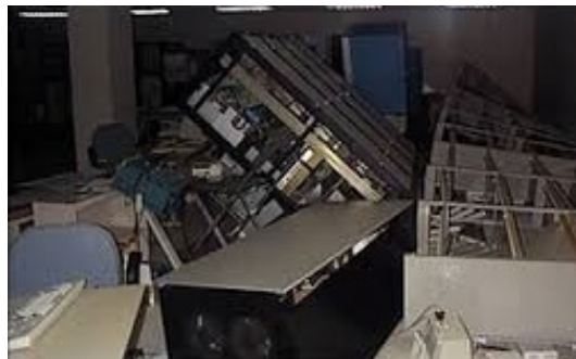
Figure 1-2. Overturned computer equipment [16]
