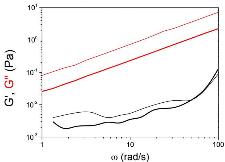
Figure 11.S9. Frequency sweeps at constant strain for propiolate-PDMSs **2** (thick line) and **3** (thin line).
