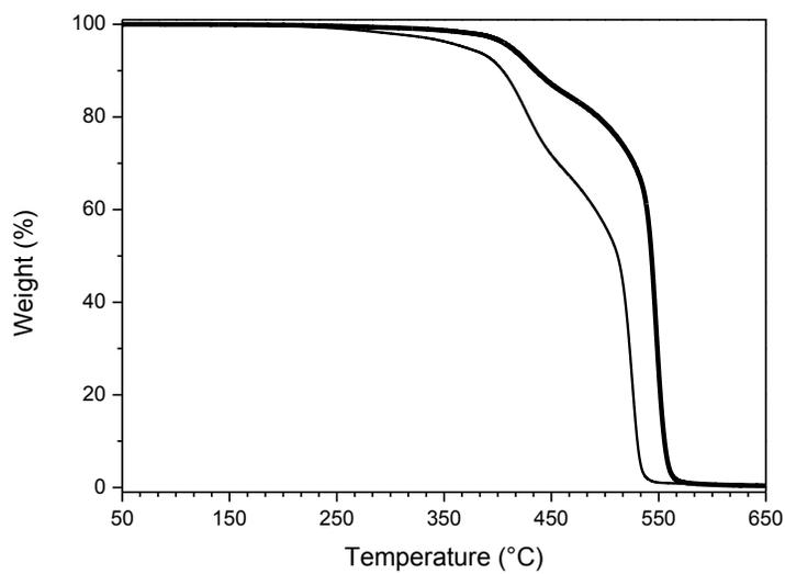
Figure 11.S8: TGA of 4 (thin line) and 5 (thick line) elastomers.
