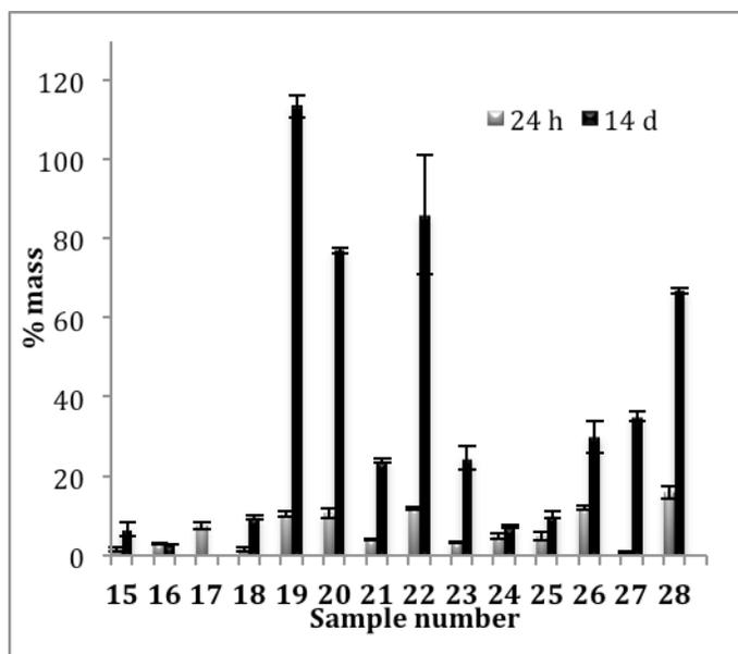
Figure 9.5S: Water uptake (wt%) at 24 hours and 14 days
