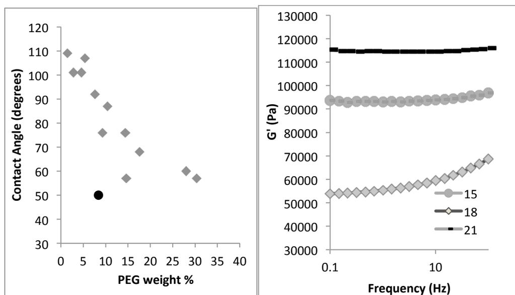
Figure 4.3: A Left: Contact angle vs. PEG weight percent (The outlier (•) represents the wettable elastomer **25**) B Right: Example storage modulus of elastomers/gels.
