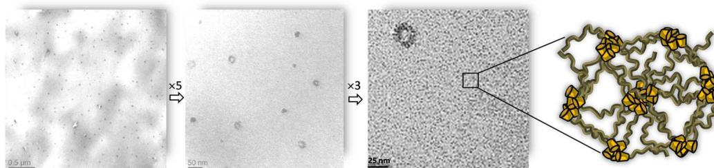
Figure 6.4: TEM images ( $\text{RuO}_4$  stain) of microtomed **4** elastomer at three increasing zooms (see scale bars on photos). The PDMS material is strengthened by big aggregates (around 40 nm in size) and tightened by numerous small clusters (of about 2 to 5 nm). Right: schematized networks formation by CD clusterization.
