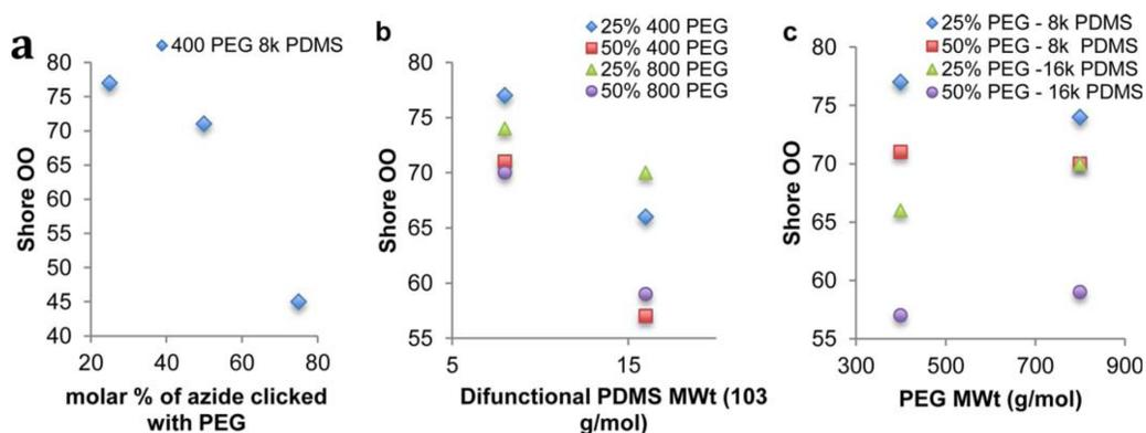
Figure 4.2: Changes in elastomer hardness: a) as a function of the quantity of grafted PEG, b) with increasing difunctional PDMS molecular weight, c) with increased PEG molecular weight.
