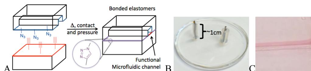
Figure 5.1: A: Schematic of adhesion of functional PDMS B: Elastomer 5 showing inserted tubing with wire and C: colored water through the channel
