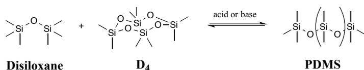
Figure 1.2: Equilibration reaction to grow PDMS chains
