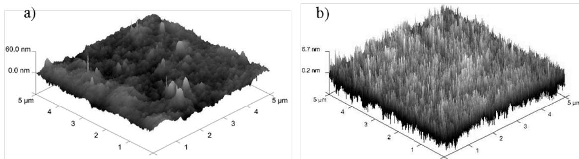
Figure 9.6S: AFM of rubbers **22** (a)  $R_q = 6.7$  and **25** (b)  $R_q = 1.9$
