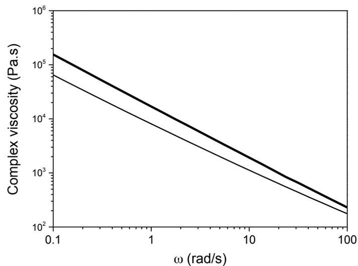
Figure 11.S11. Complex viscosity versus angular frequency for elastomers 4 (thick line) and 5 (thin line).
