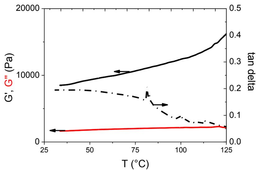
Figure 11.S10. Temperature sweeps at constant strain for elastomer **4**.
