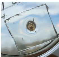
Figure 10.S1: Huisgen bonded interface after the delamination experiment, star/fissure cracks through the material (background, sky)
