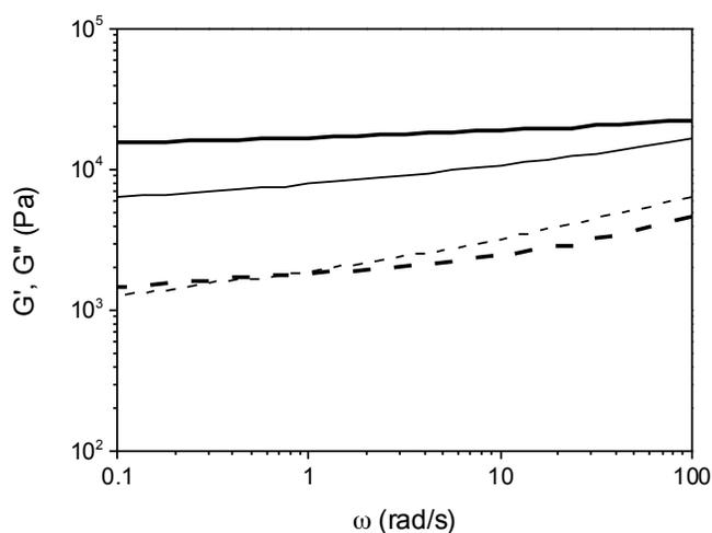
Figure 6.3: Frequency sweeps rheology measurements, giving  $G'$  (solid lines), and  $G''$  (dot lines) for **4** (thick lines) and **5** (thin lines).
