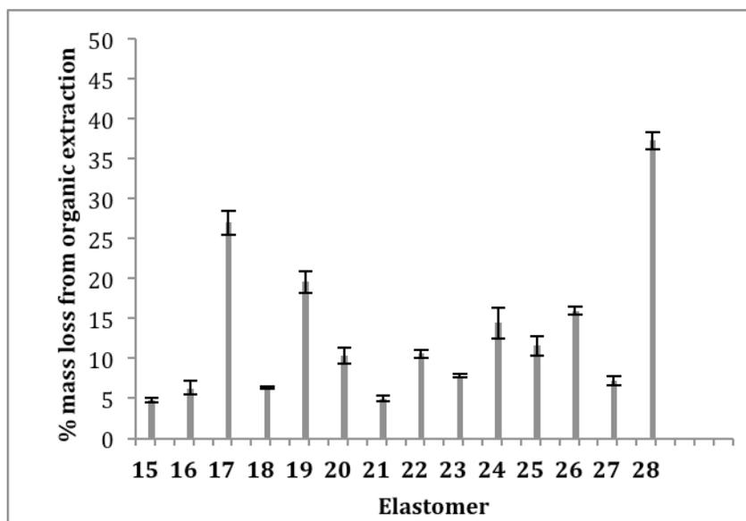
Figure 9.3S: Organic extractables from the elastomers.
