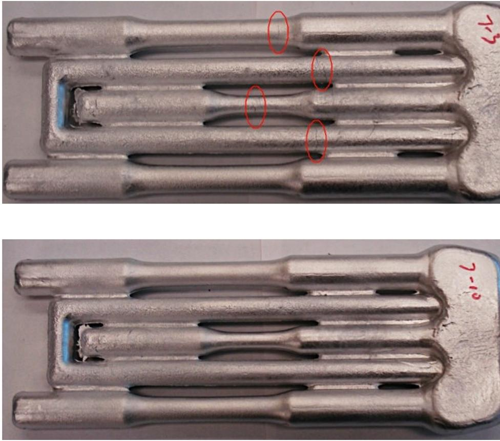
**Figure 5-1 Image showing the typical appearance of the alloy castings (a) without the TiBor addition (Alloy 7) and (b) with the TiBor addition (Alloy 7) Red frames document the locations of visible cracks.**
