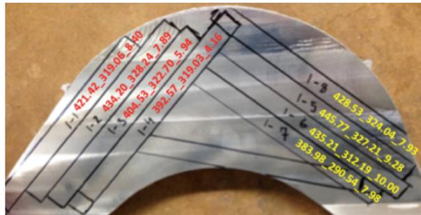
Figure 4-6 Locations of the tensile samples cut from the camber link.
