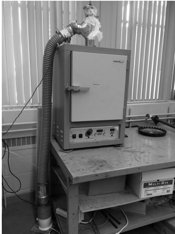
Figure 3.4. Makeshift apparatus used to control temperature and humidity settings for short term environmental stress cracking tests.
