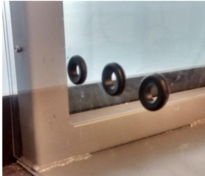
Figure B-6: Wire Ports in Back of Test Chamber
