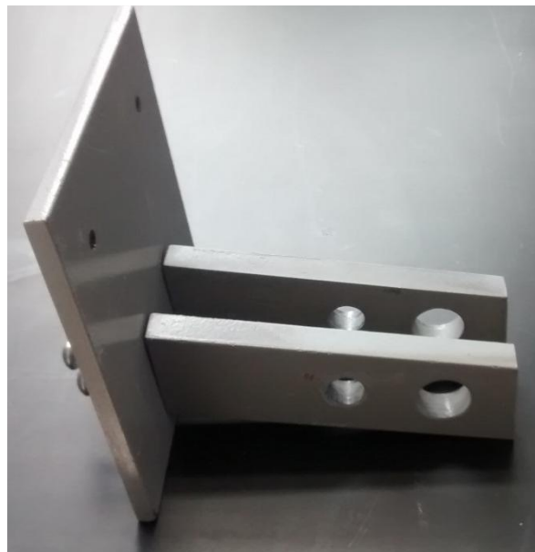
Figure B-3: A Close-Up View of an Example ATD Bracket
