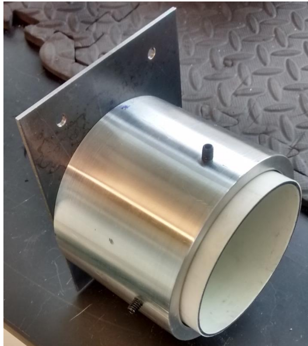
Figure B-2: A Close-Up View of the Cadaveric Specimen Bracket with a 4" PVC Section Secured in Place
