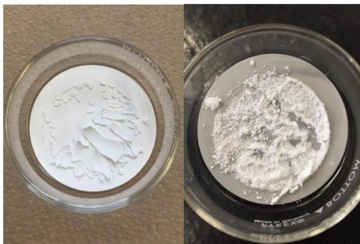
**Figure 2.9.** Dried samples of the instantaneous mixing (left) and slow mixing (right).
