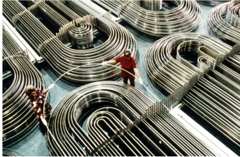
Figure 2.12: Main internal structure in steam generator is a series of parallel inverted U-tubes.
