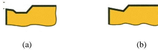
Figure 16: Chip Breaker profile: (a) CNMG432 (b) CNMP432
