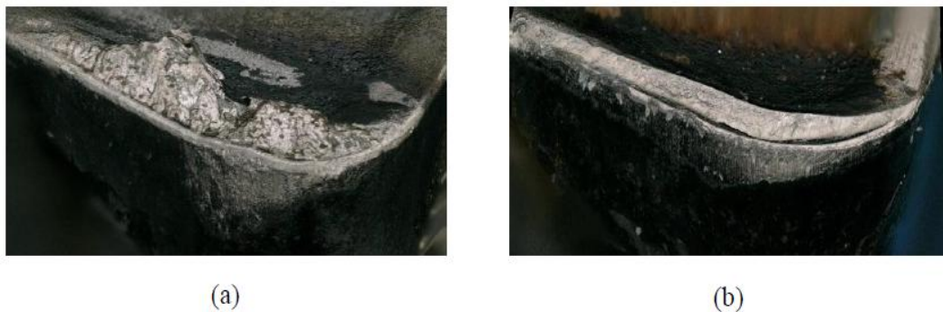
Figure 44: 3D images of worn tool after 3000 m cut: (a) uncoated insert (b) CrN/WN coated insert
