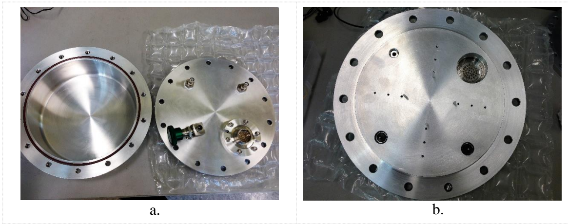
Fig. 2.3 a. Fabricated detector chamber lid and air side of the baseplate, b. Fabricated detector chamber baseplate (vacuum side)
