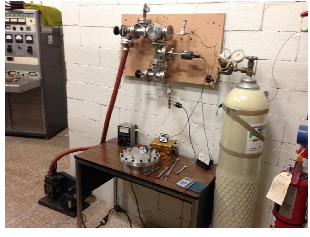
Fig. 2.18 Vacuum pump and filling gas station
