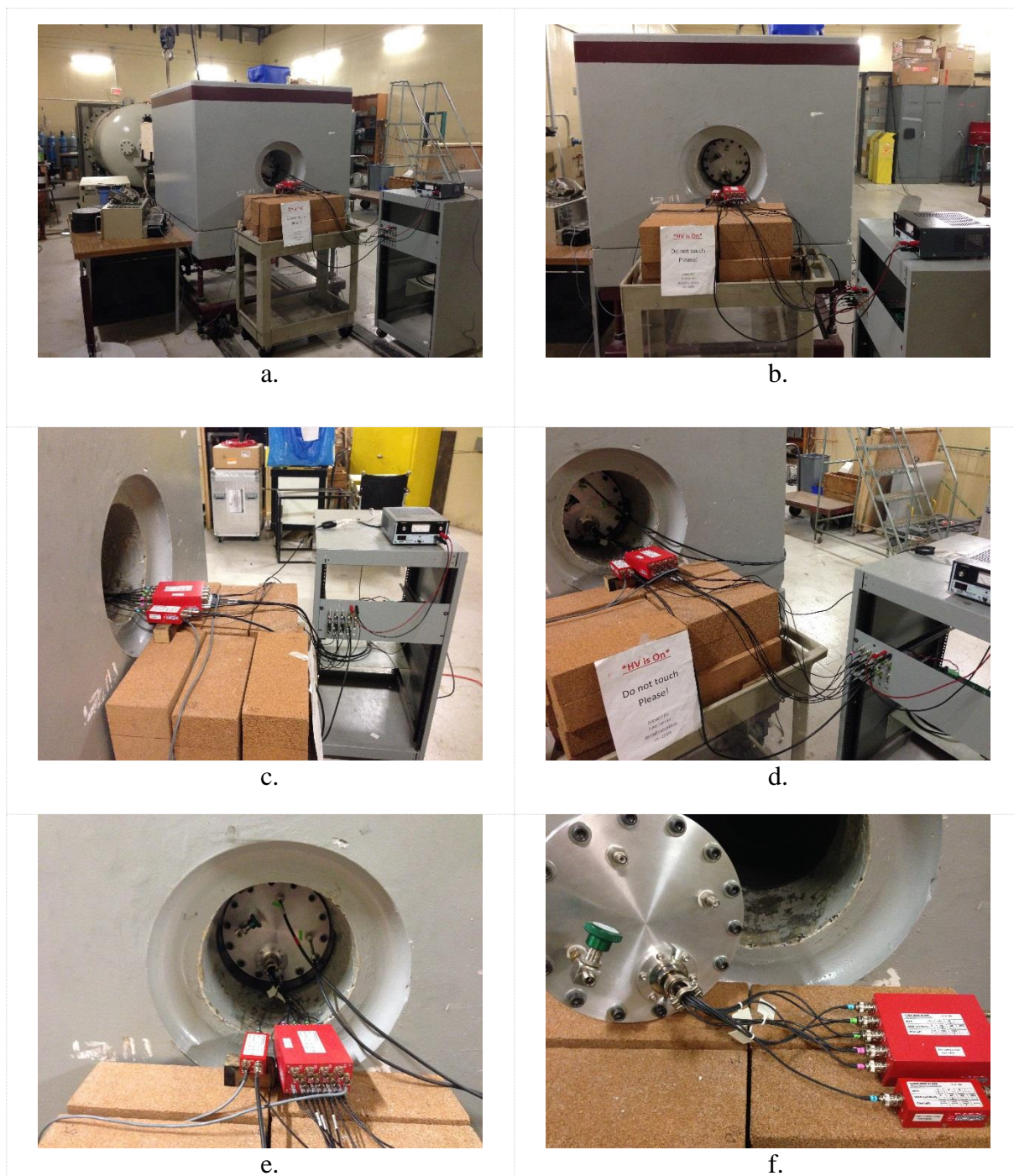
Fig. 4.7 Experimental setup for multi-volume detector and multi-input MMI-DSP: 2D THGEM detector is placed in the irradiation cavity and connected to CAEN 8 channels and 1 channel charge sensitive preamplifier
