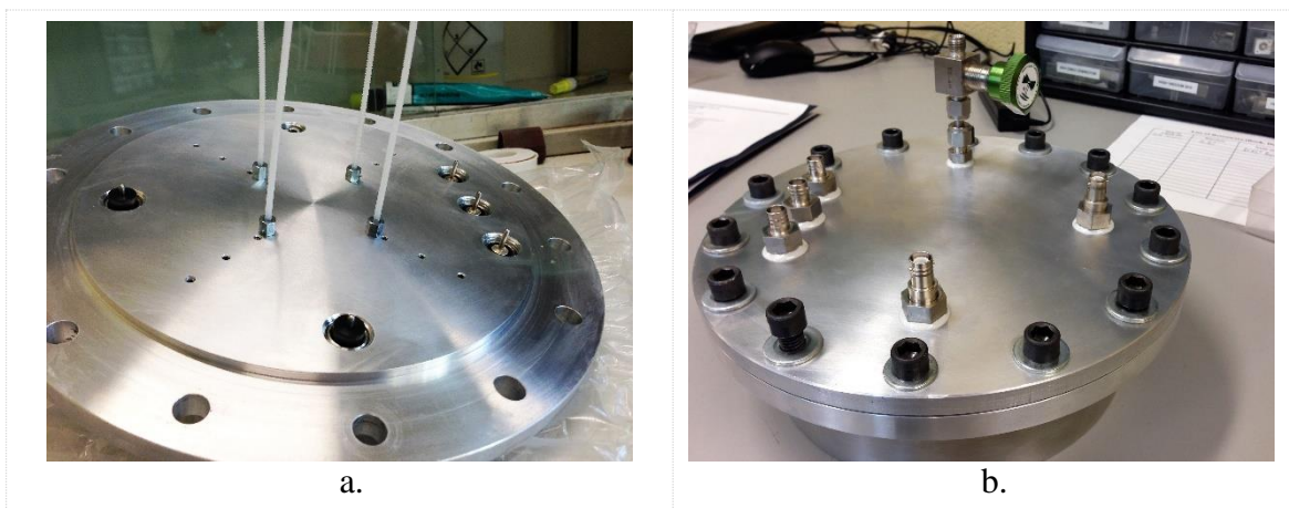
Fig. 2.4 a. Fabricated detector chamber baseplate with 3 signal inputs (vacuum side), b. Assembled detector chamber with 3 signal inputs
