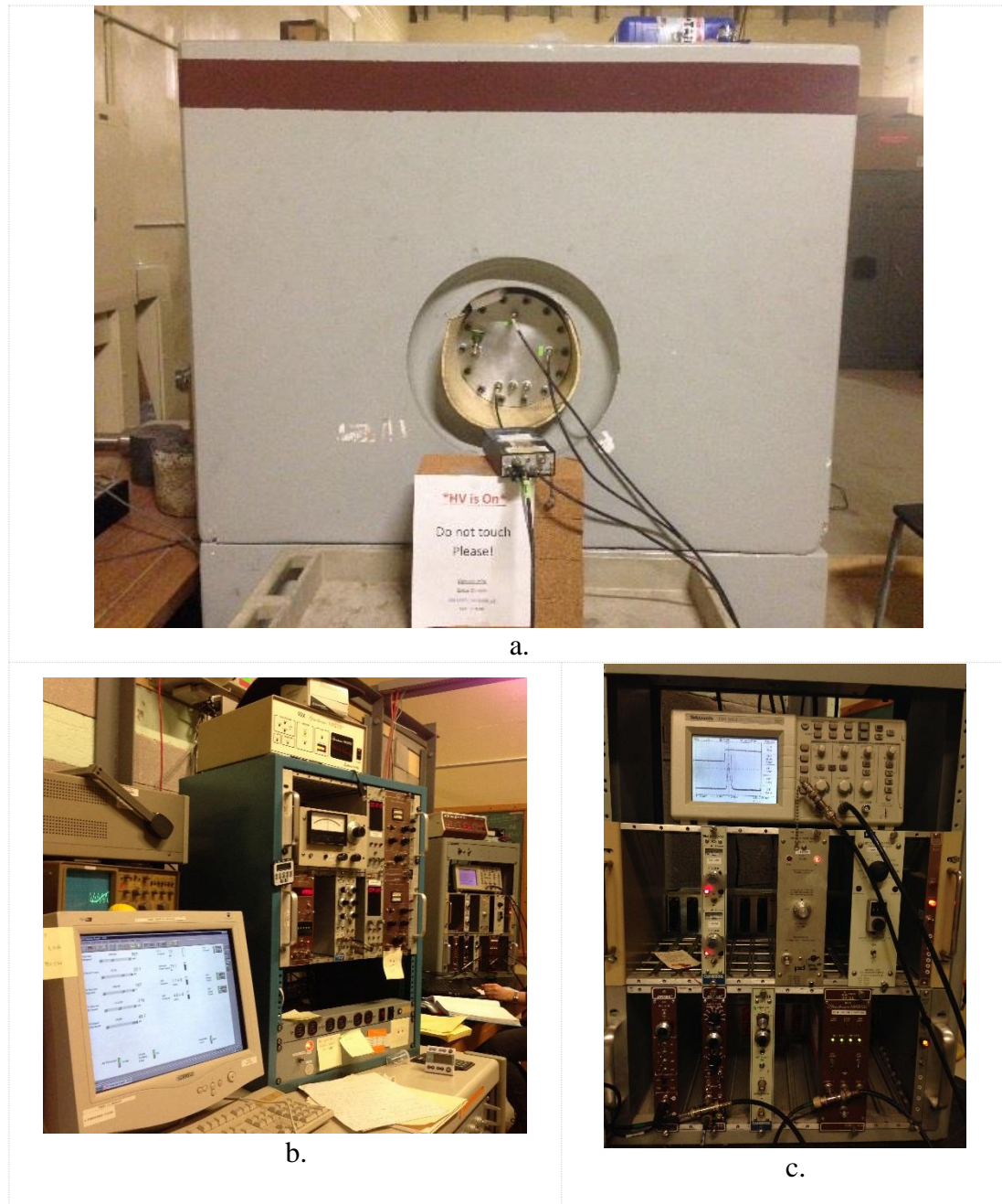
Fig. 4.4 a. Single volume detector placed in the irradiation cavity connected to the ORTEC charge sensitive preamplifier, b. Control room: accelerator operator desk and electronics c. electronics NIM bin: dual HV, pulser, amplifier
