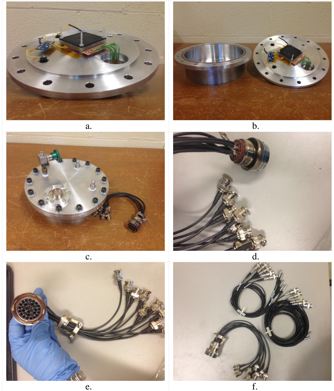
Fig. 2.14 a. & b. A 2-dimensional multi-volume detector assembly, c. sealed and closed detector, d. & e. Multi-pin plug (RG-170 cable soldered to the pin and inserted into the plug), f. custom made required signal cables: multi-pin plug – 9 BNCs, 9 signal cables LIMO – BNC
