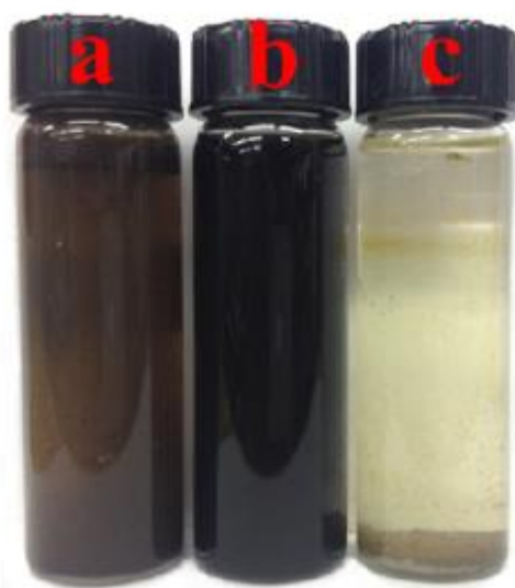
Figure 7-2 Sedimentation test in a mixed ethanol (50%) – water (50%) solvent, containing 1 g L -1 LG and (a) 4 g L -1 MnO 2 (b) 1 g L -1 MWCNT (c) 2 g L -1 MnO 2 and 0.5 g L -1 MWCNT
