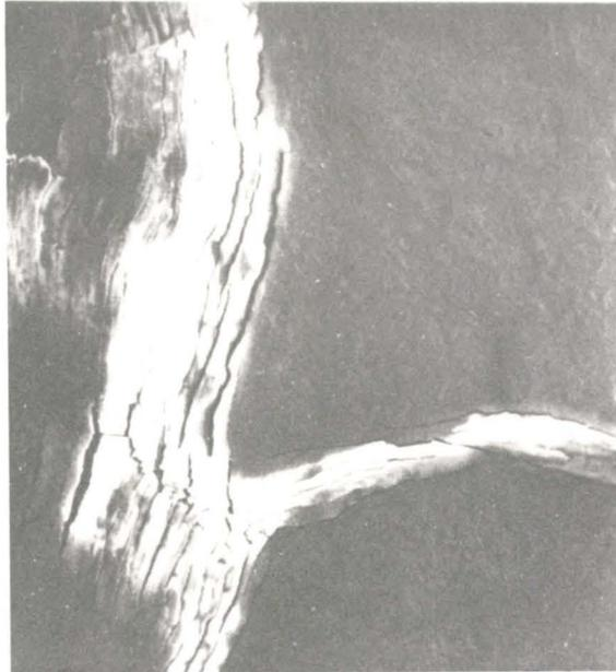
Figure 11. Topography of Sample Oxidized at  $991^{\circ}\text{C}$  for 12 hours. (Magnification 20X)
